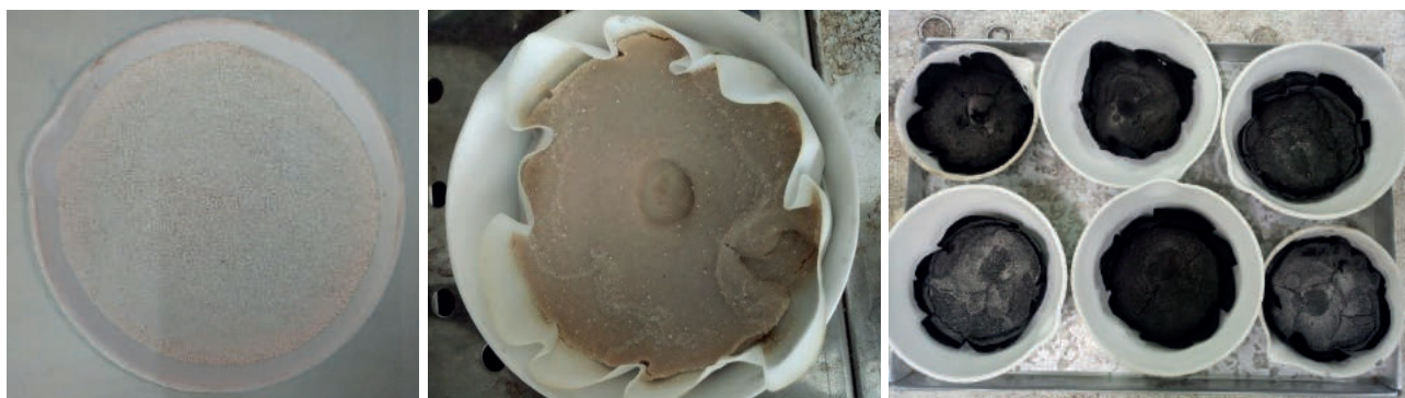
FIGURE 6: Appearance of carrageenan filter cake (a) before hydrolysis (b) after filtration (c) after drying at 105°C for 24 hours.
