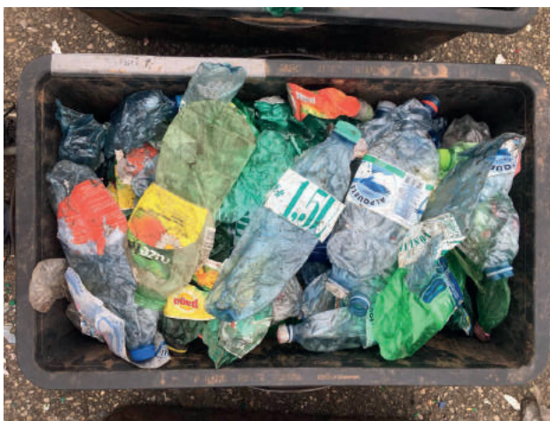
FIGURE 1: Input material for delabelling trials - PET bottles from the public collection system.
