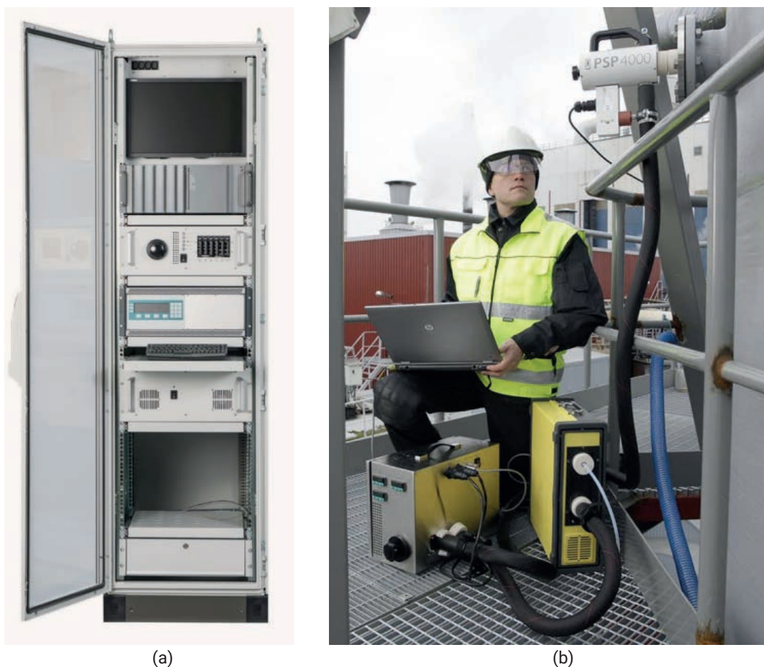
FIGURE 1: FTIR technology applications: (a) Gaset CEMS IIe; (b) Portable DX4000 measuring system.
