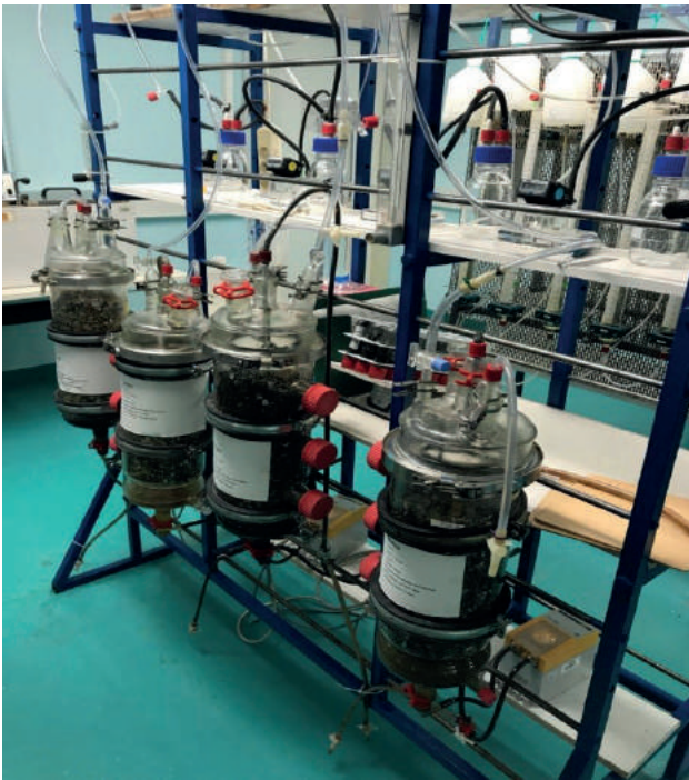
FIGURE 1: Setup of Landfill simulation reactor experiment.
