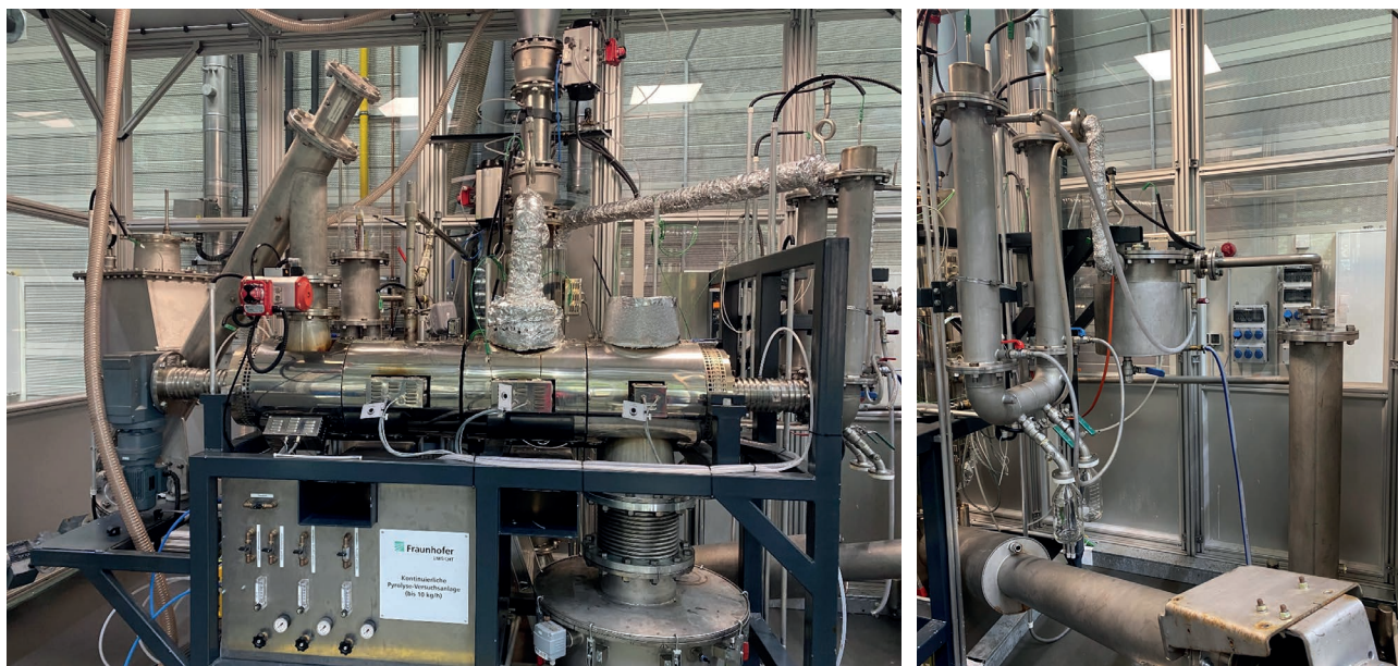
FIGURE 1: Picture of the pyrolysis plant combined with the chlorination reactor.
