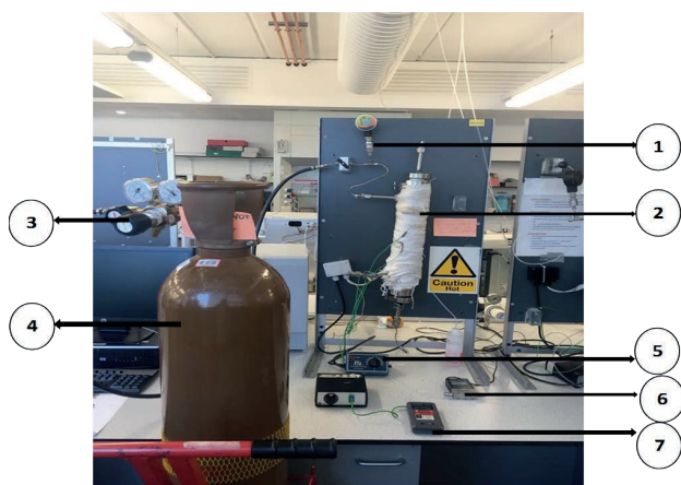
FIGURE 1: Experimental set-up showing all equipment including; pressure gauge(1), membrane module covered with heating tape(2), gas regulator(3), gas cylinder(4), heat regulator(5), volumetric meter(6) and temperature indicator(7).
