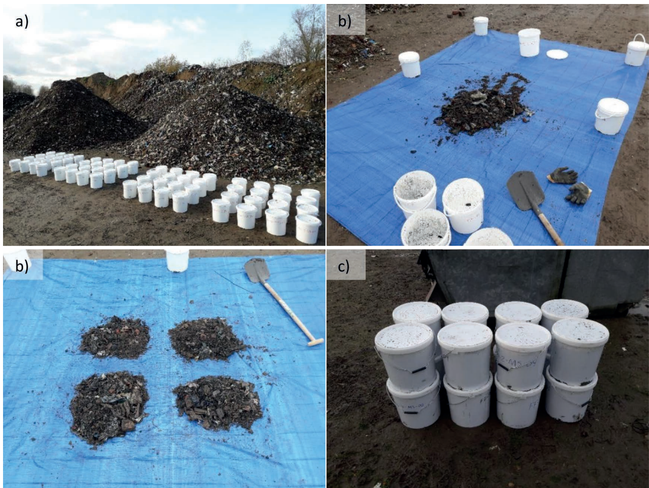
FIGURE 4: a) Single samples, b) quartering method and c) composite samples.
