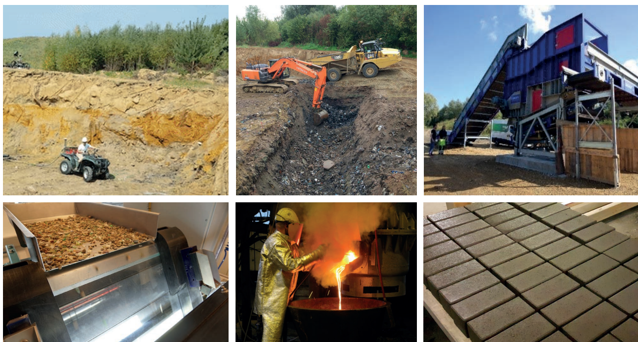
FIGURE 2: Overview of key aspects of the NEW-MINE value chain. Upper part from left to right: Geophysical exploration, excavation and ballistic separation at the Mont-Saint-Guibert landfill in Belgium. Lower part from left to right: sensor based sorting, tapping of slag derived from gasification of the calorific fraction derived from EFM, pavers produces using an inorganic polymer derived from EFM SLAG. Pictures from C. Bobe, C. Garcia Lopez and J.C. Hernández Parrodi.
