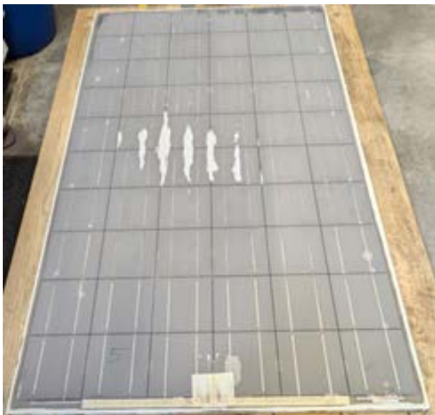
FIGURE 1: The PV panels pre-treated with a sanding process to remove the backsheet.
