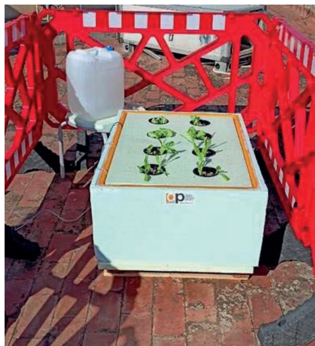
FIGURE 1: The examined hydroponic green roof system.
