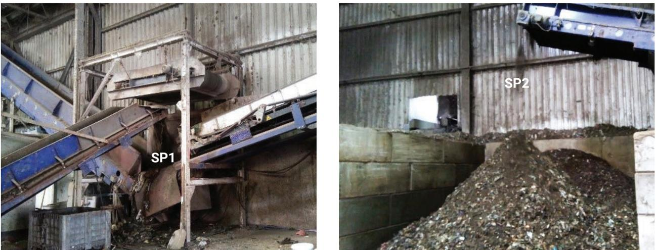
**FIGURE 6:** Input material after a shredder and an overbelt magnet, SP1 (left) and fines from the first screen 60 mm, SP2 (right).
