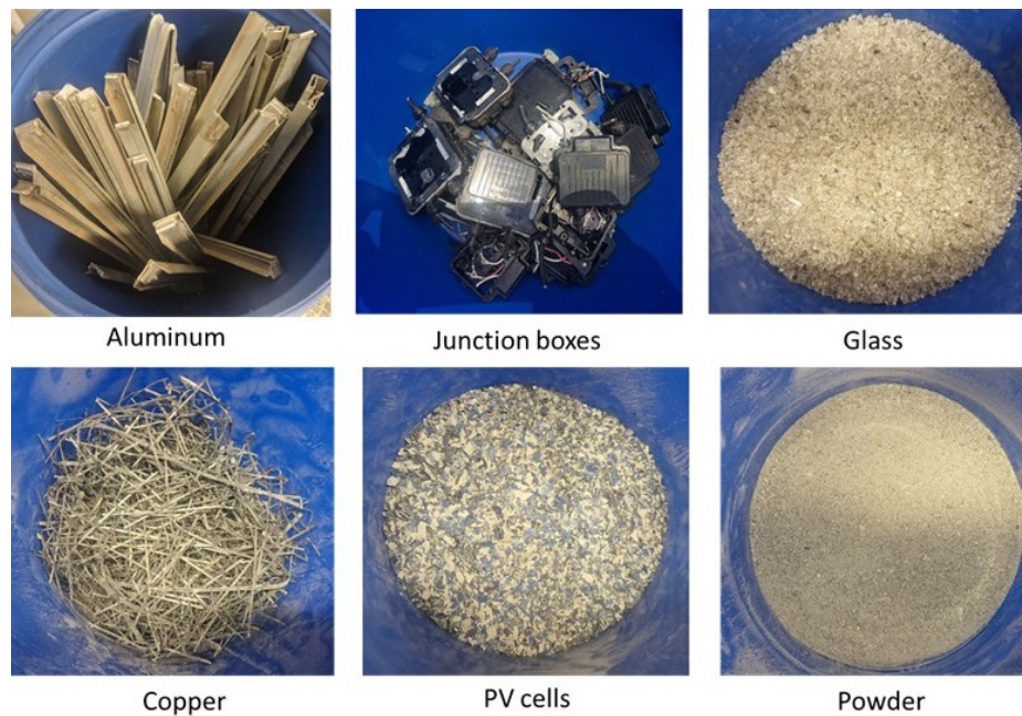
FIGURE 7: Materials recovered in the pilot plant performing thermomechanical recycling.
