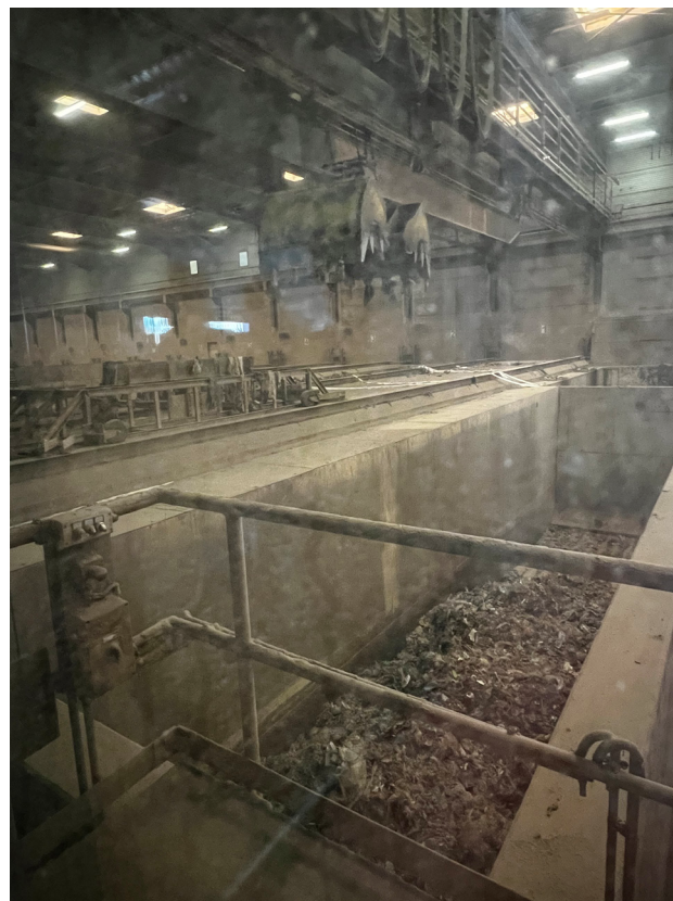
FIGURE 5: Biological drying stabilization. Source: Author's personal collection, 2023.
