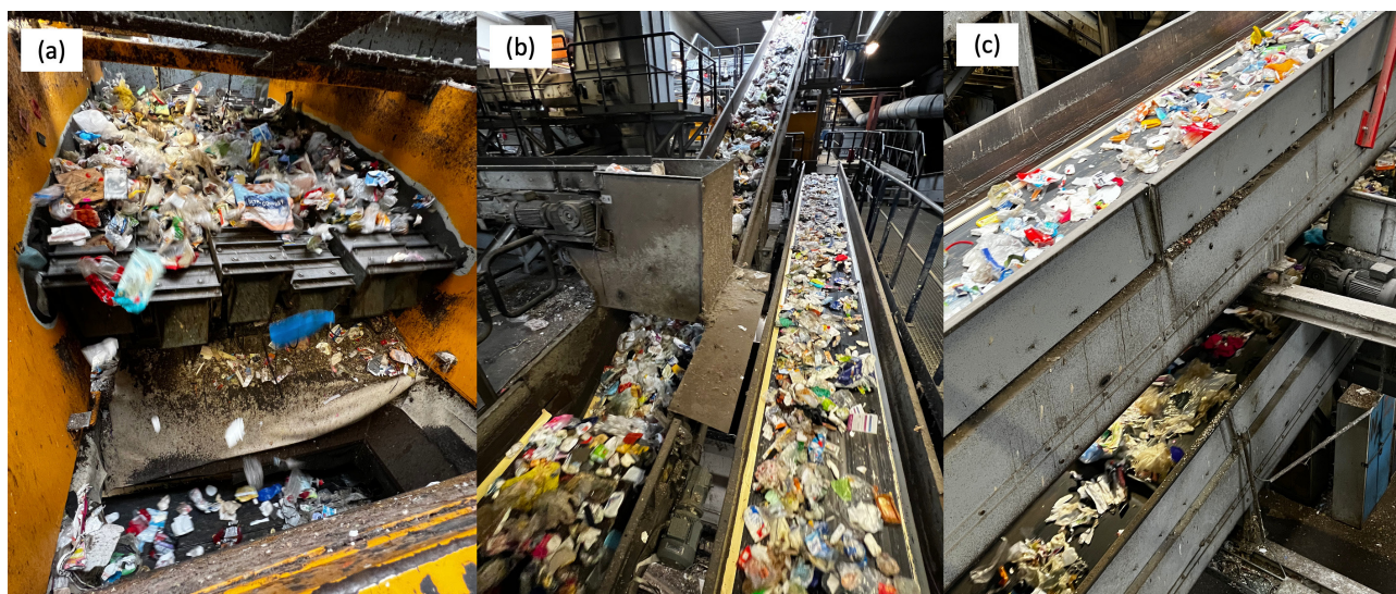
FIGURE 4: Operation flow: (a) waste separation by ballistic separator; (b) reallocation of light and heavy materials on two different belts; (c) separation of reusable materials for recycling and non-recyclable materials for incineration. Source: Author's personal collection, 2023.
