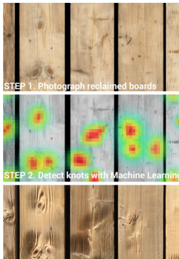
FIGURE 5: Machine Learning application for reclaimed wood knot automated detection (source: https://www.architectmagazine.com/project-gallery/embody-computation-lab_o ).
