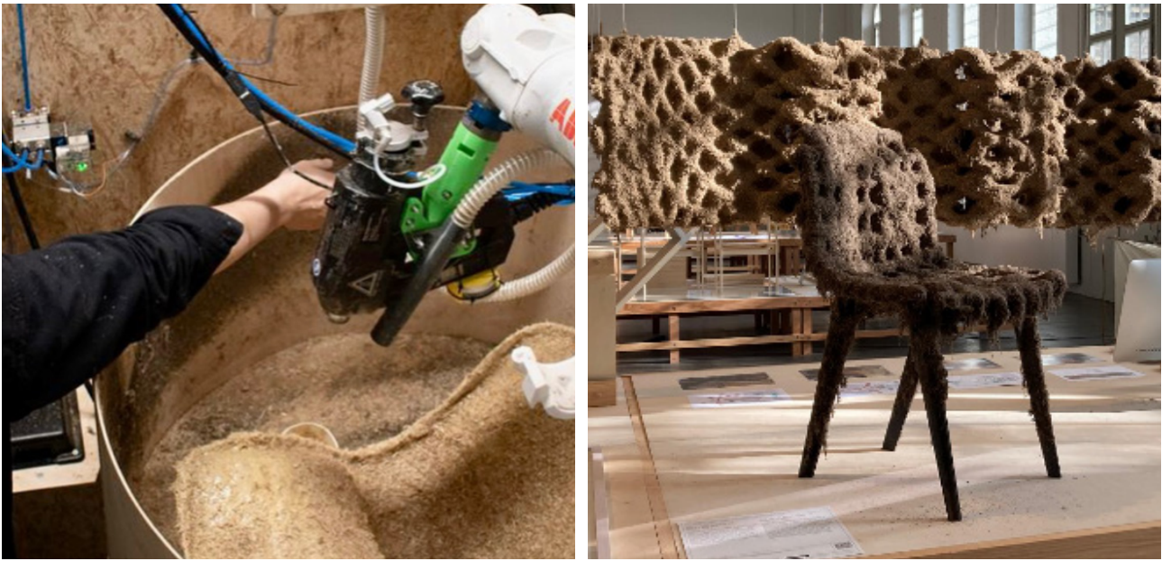
FIGURE 8: Process and prototyping of a “3D sprayed” chair, developed at Center for IT in Architecture, Royal Danish Academy, Copenhagen (DK).
