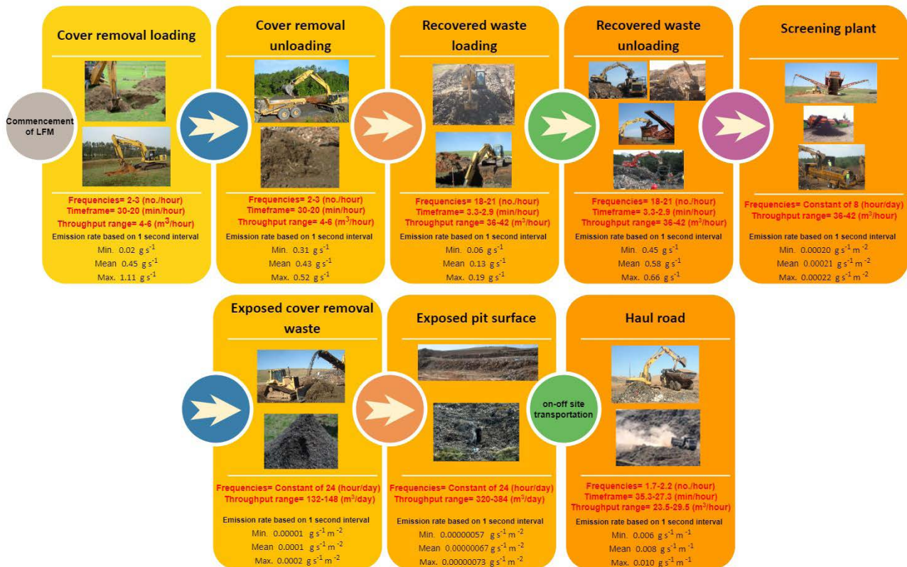
FIGURE 8: Flowsheet illustrating LFM processes and defining volumetric throughput, number of loading frequencies and timescales ranges for each unit operation with their respective emission rate.
