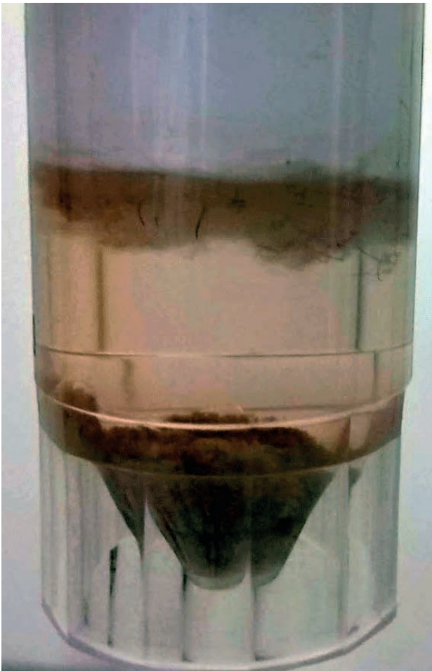
FIGURE 1: Partially floating quartz sand commingled with added polyester fibres and polypropylene granulate (model mixture) after sink-float separation in a heavy liquid; separation efficiency poor although accurate adjustment of density.
