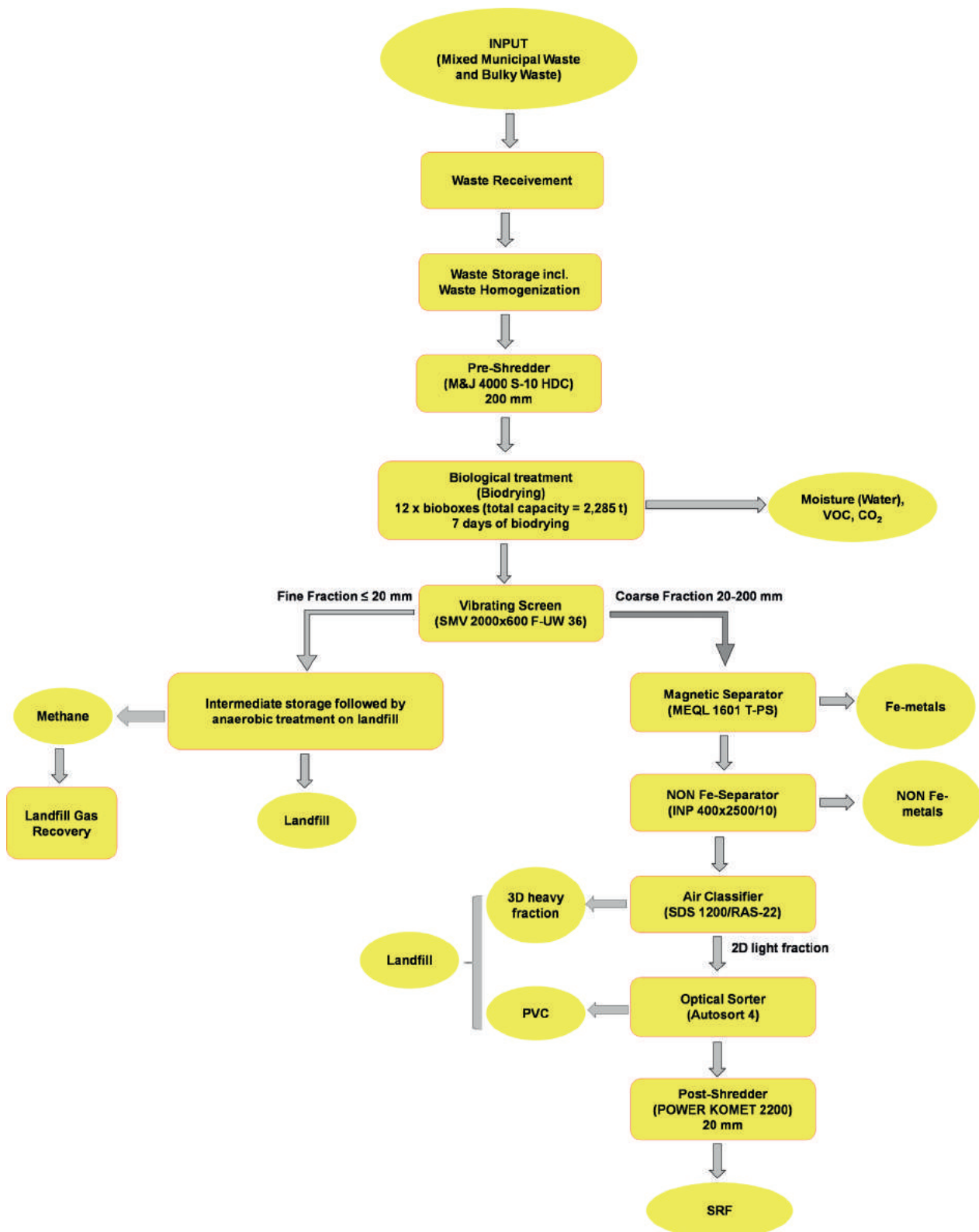
FIGURE 2: Multistage processing scheme as an example of a SRF production Plant Type #1.
