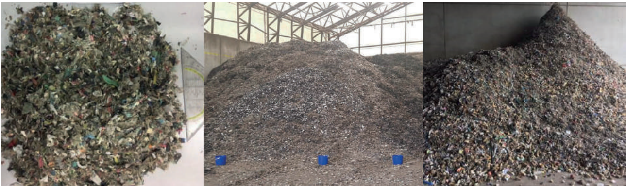
FIGURE 7: Photo documentation of the investigated SRF from Plant Type #1 (left), Type #2 (middle) and Type #3 (right).
