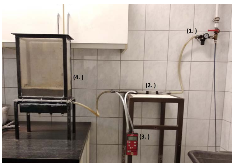
FIGURE 2: Laboratory scale test equipment (1 pressure regulator, 2 Venturi tube, 3 differential pressure meter, 4 laboratory model fluidised bed reactor).
