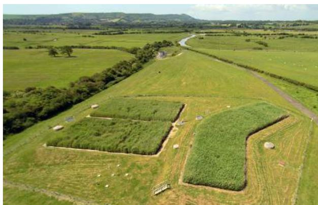
**PLATE 2:** Aerial view of the vertical flow reed bed, and the two parallel horizontal flow reed beds, following construction by Phoenix Engineering in 2010.
