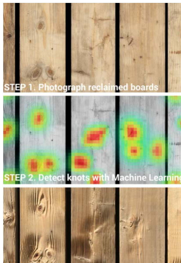
FIGURE 5: Machine Learning application for reclaimed wood knot automated detection (source: https://www.architectmagazine.com/project-gallery/embodyed-computation-lab_o ).
