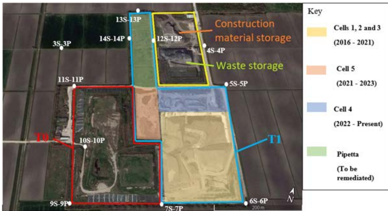
FIGURE 1: Map of Villadose landfill showing Taglietto 0 (T0), Taglietto 1 (T1) and its landfill cells, the temporary waste storage area the storage area for construction materials and the locations of the pairs of piezometers. T2 and T3 are not visible as they are located a few hundred metres from T0 and T1.
