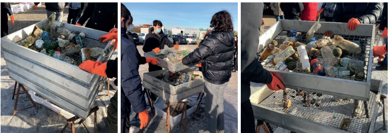
FIGURE 5: System of sieves of different side mesh (200, 100, 80, 50 and 20mm) used for granulometric analysis.
