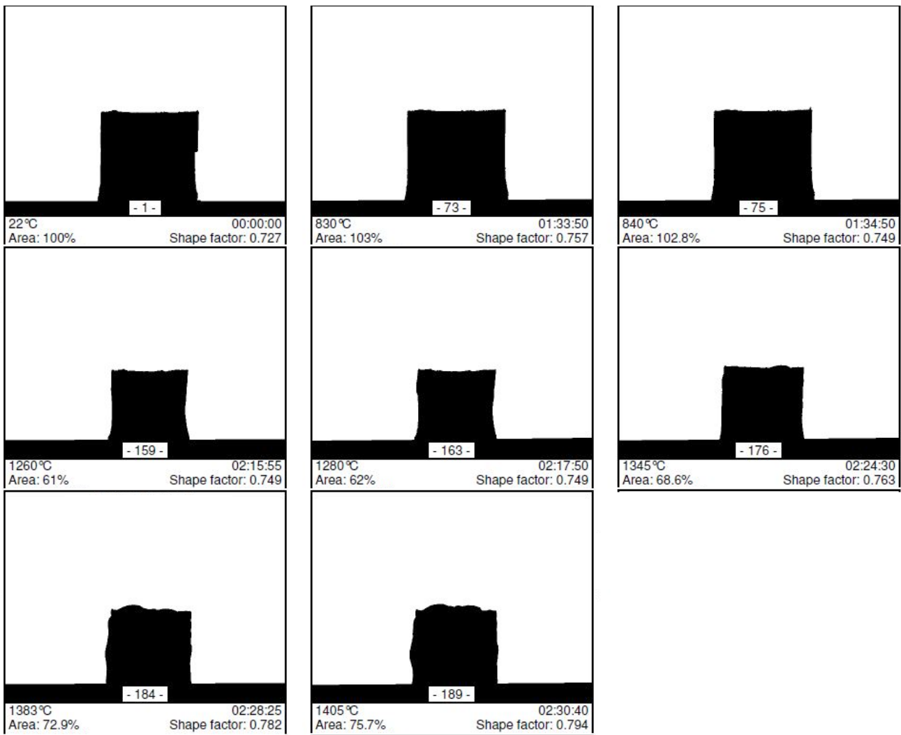
FIGURE 4: Images of changes in sample profile shape in line with measurements taken under the heating microscope.
