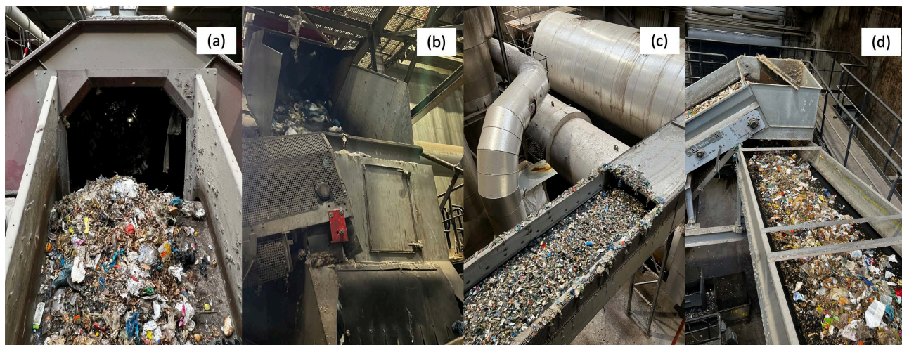
FIGURE 3: (a) material sorting by granulometry; (b) metal separation; (c) crushing; (d) drying. Source: Author's personal collection, 2023.
