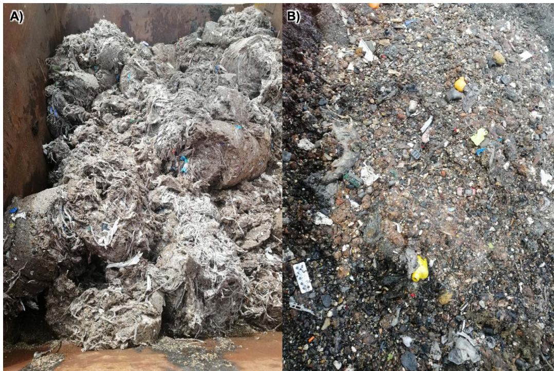
FIGURE 1: Discarded waste from the preliminary stage. A) Fibrous waste; B) Grit removed.
