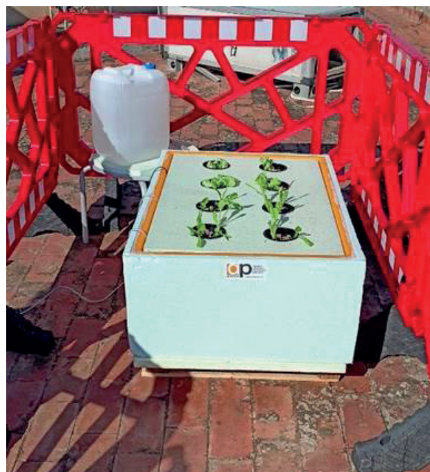
FIGURE 1: The examined hydroponic green roof system.
