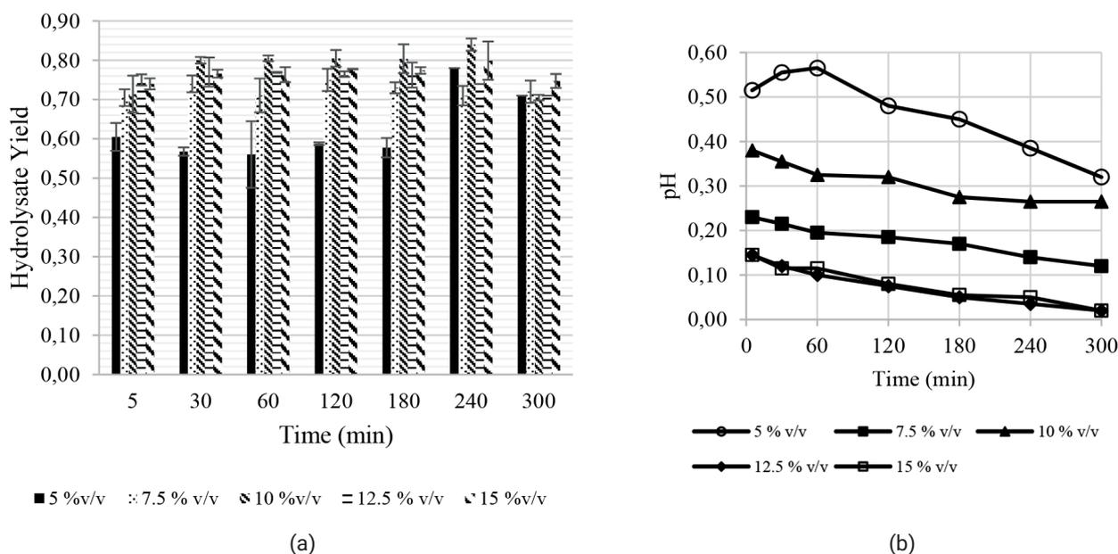
**FIGURE 3:** Hydrolysate yield (a) and pH (b) of hydrolysates at constant temperature and SSR of 95° C and 8 mL/g, respectively, and varying acid concentration (5 % v/v to 15 % v/v) and reaction time (0 to 300 min).
