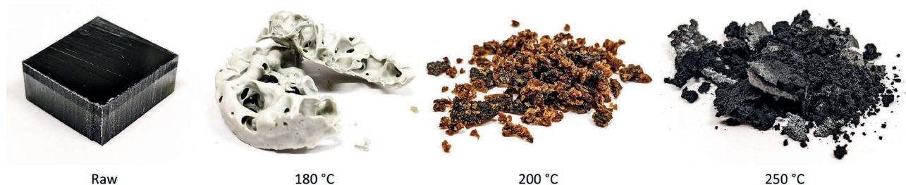
FIGURE 2: Appearance of CDA and of the solid products obtained at different HTC temperatures.
