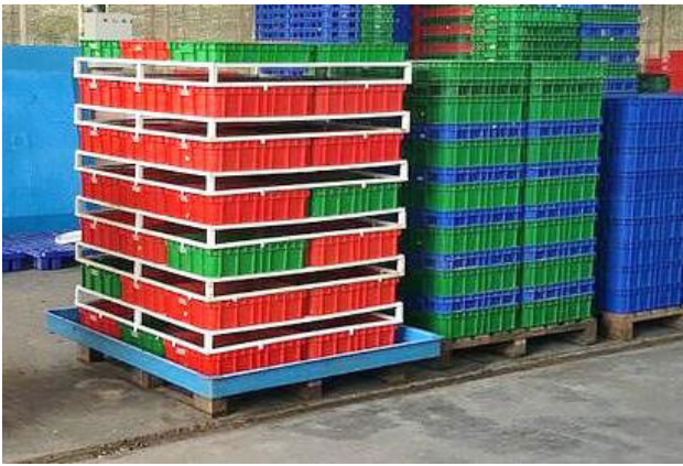
FIGURE 2: Stack of larvero containers with ventilation frames in-between levels (Dortmans et al, 2017).
