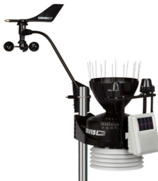
FIGURE 1: Monitoring system: a. Ellona outdoor electronic nose and b. Davis Instruments, Vantage Pro2 meteorological station.
