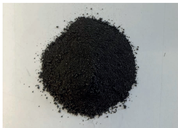
FIGURE 2: Teesside sample No. 1 after sieving through 2 mm mesh.
