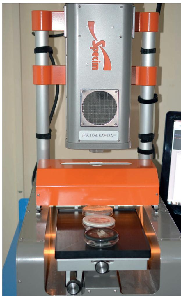
**FIGURE 2:** A schematic image with a picture of SisuCHEMA XL™ Chemical Imaging Workstation (Specim, Finland).
