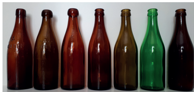
FIGURE 1: The development of the standardized 33 cl Stockholm bottle over 130 year. The two left bottles were blown by hand (1880s, 1901) and the three bottles on the left (1880s, 1901, 1930) were sealed by a cork. The others were blown by a machine and capped (1937, 1959, 1968, 2013). Image used with permission from Henriksson (2019).
