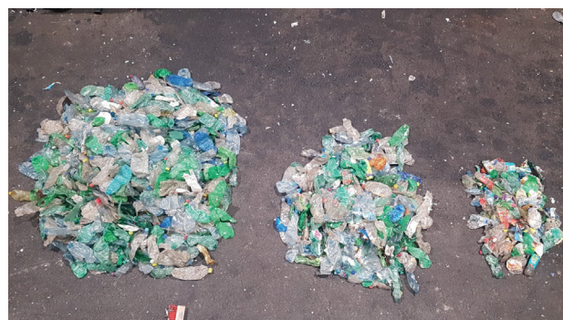
FIGURE 3: Output fraction of the delabeller - from left to right: category 1 (Good), category 2 (Middle), category 3 (Bad).
