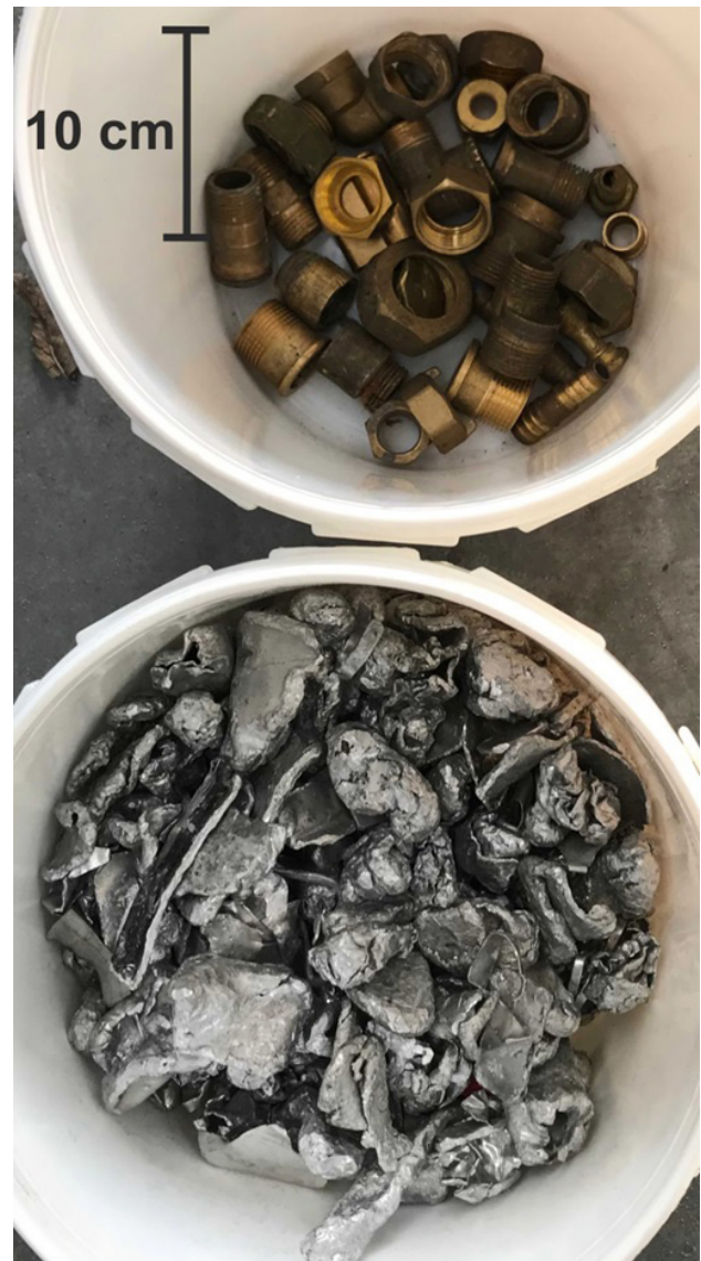
FIGURE 9: (Left) Feed of pilot experiment (30–100 mm copper-aluminium scrap); (Right) Products of pilot experiment (Al and Cu products).
