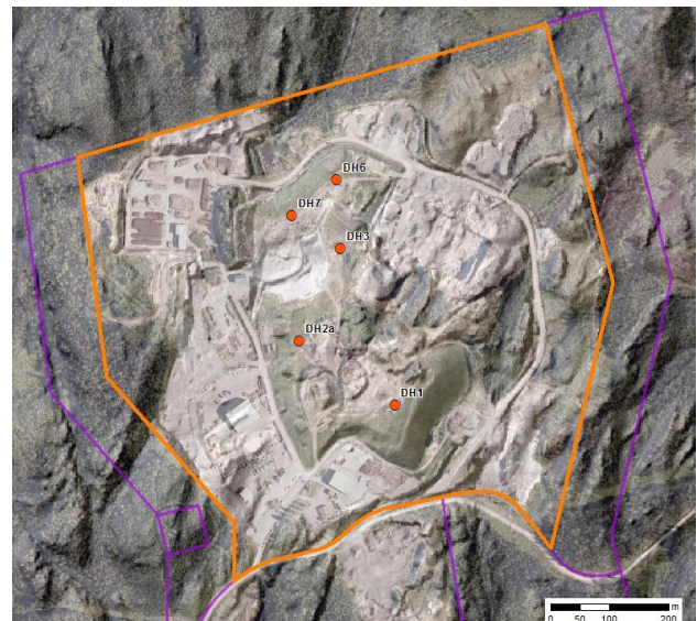
FIGURE 1: Topographic map of Metsäsairila MSW landfill site obtained using laser scanning based DEM with 2 metres resolution overlaid with aerial photography (orange dots: location of the sampling points).
