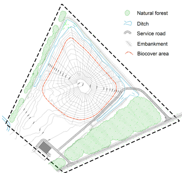
FIGURE 5: Layout of a remediated landfill as initially proposed (Kriipsalu et al., 2016).
