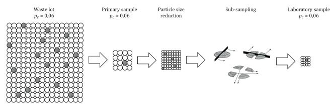
FIGURE 2: Graphical representation of the ideal process for decreasing the size of samples.
