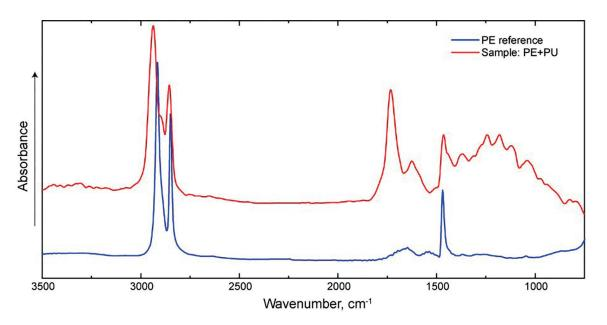
FIGURE 5: PE spectra. Spectrum of a reference material (blue) and PE particle spectrum acquired with FT-IR microspectrometer (red); spectra are shifted on the y axis for clarity.
