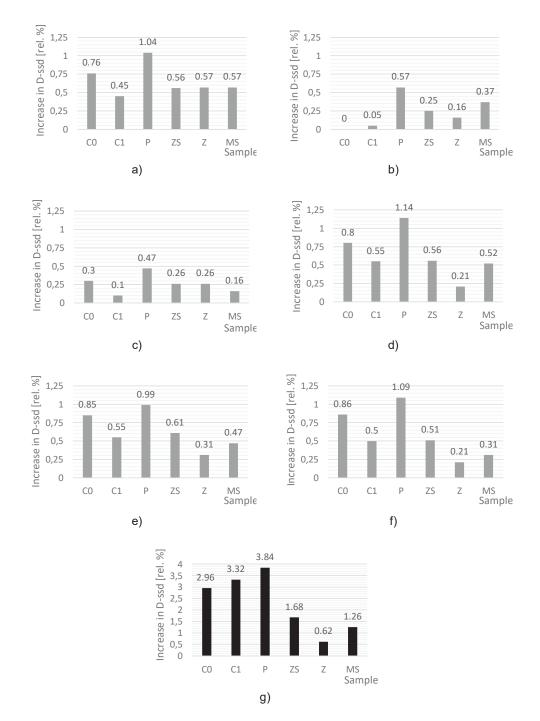
**FIGURE 5:** Changes in bulk densities of cement pastes after exposure to a) Ca(OH)2 reference medium, b) deionized water, c) natural acid rain, d) model acid rain with pH = 6, e) model acid rain with pH = 4, f) model acid rain with pH = 2, g) model acid rain pH = 2 - samples with precipitates.
