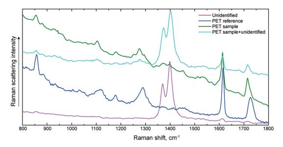
FIGURE 3: Raman scattering spectral analysis results. Results for PET reference material (blue); undefined spectrum (pink), PET particle in the sample (green), and PET with undefined spectra (cyan); spectra are shifted on the y-axis for clarity.
