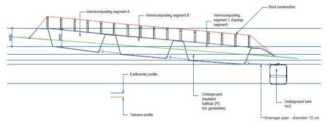
FIGURE 1: Pilot-scale vermicomposter scheme (if not directly specified, the dimensions are given in cm).
