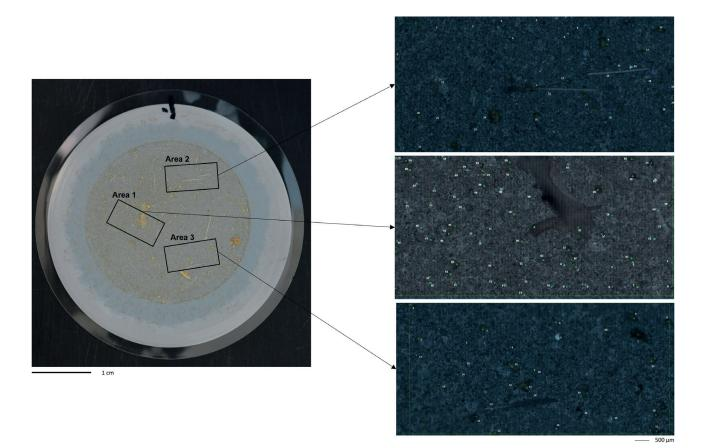
FIGURE 2: Example of mapping areas. Mapping areas within sample 8 with measurement points on randomly selected particles highlighted on the right (70 points in total).
