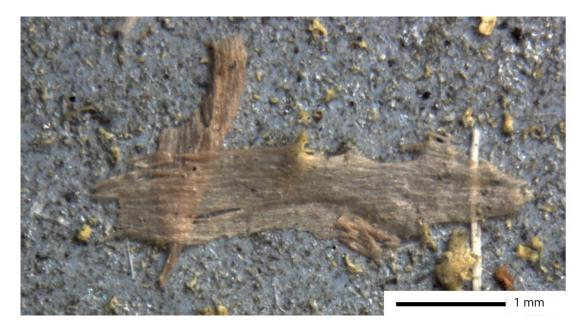
FIGURE 4: PE particle in sample 8. The PE particle image acquired with stereomicroscope Lecia M205 C with x1.25 magnification.
