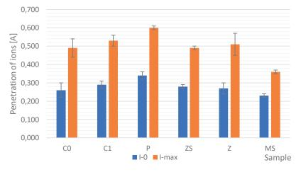
FIGURE 3: Results of the RCP test of cement pastes before the corrosion experiment...
