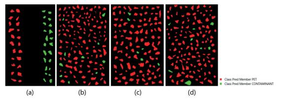
FIGURE 5: Full spectrum PLS-DA prediction maps for the validation (a), test 1 (b), test 2 (c) and test 3 (d) datasets.
