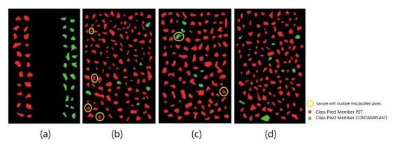
FIGURE 8: VIP prediction maps for the validation (a), test 1(b), test 2 (c) and test 3 (d) datasets.
