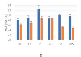
**FIGURE 6**: Comparison of absorption of cement pastes before and after exposure to a) reference medium Ca(OH)2, b) deionized water, c) natural acid rain, d) model acid rain with pH = 6, e) model acid rain with pH = 4, f) model acid rain with pH = 2.
