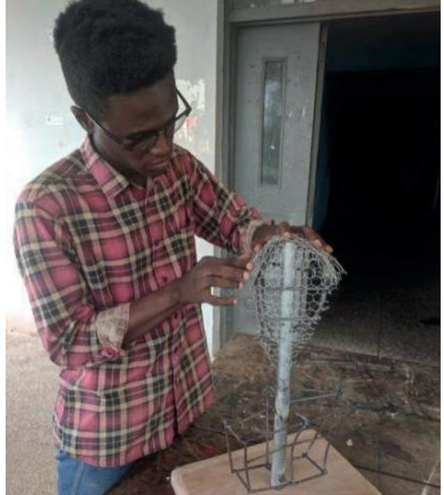
**FIGURE 26:** Wrapping the wire mesh around the armature.
