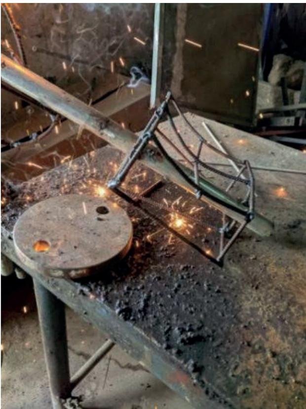
FIGURE 23: Welding the metal rods together.
