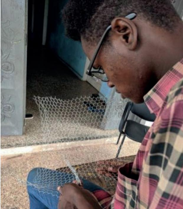
**FIGURE 25:** Cutting the wire mesh.
