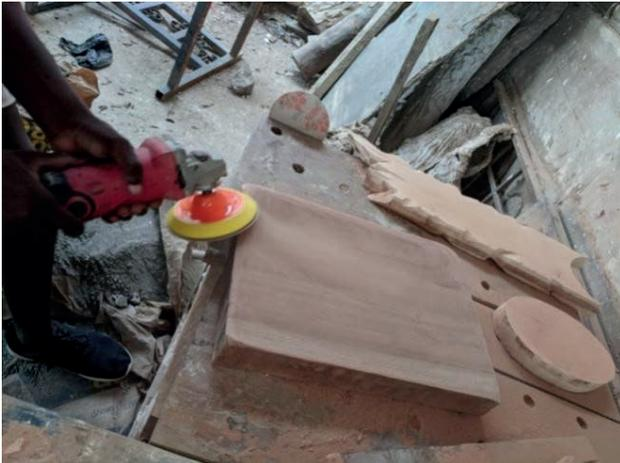
FIGURE 21: Sanding the wooden base.
