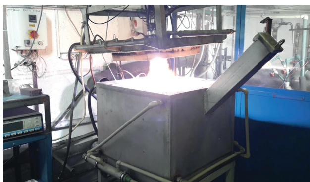
FIGURE 2: Photo of the plasmatron in operation with the reactor lid lifted.
