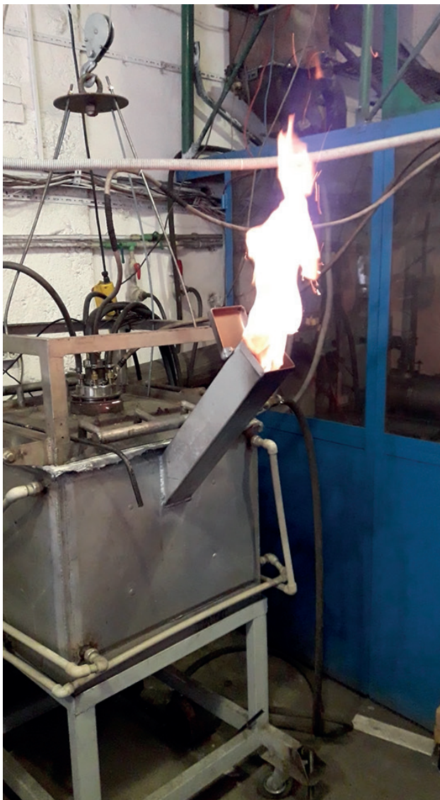
FIGURE 7: Photo of the combustible gas control flame from the pipe for supplying the WW briquettes.
