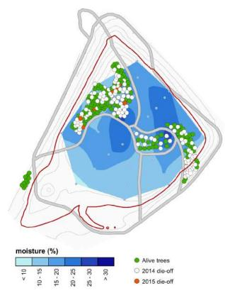
**FIGURE 9**: Tree mortality one and two years after planting, considering pH and moisture of cover layer (Tammjärv et al., 2016).
