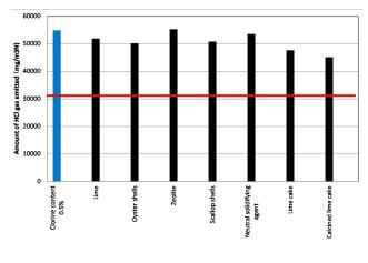
FIGURE 7: Amount of HCl gas emitted with single antichlors (waste).
