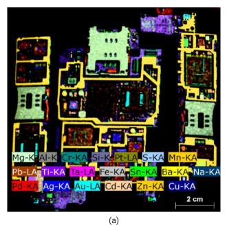
**FIGURE 4:** Hyper-map of all elements detected by  $\mu$ XRF (a) and associated average concentration of the different elements as detected by acquisition (b).
