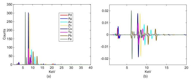
FIGURE 6: Raw (a) and pre-processed spectra (b), as resulting from the sequential application of the functions: Normalize (1-Norm, Area = 1), Baseline, Smoothing (order: 0, window: 5 pt, incl only, tails: polyinterp), 1st Derivative (order: 2, window: 7 pt, incl only, tails: polyinterp) and Mean Center.
