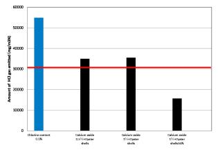
FIGURE 9: Amount of HCl gas emitted with mixed antichlors.
