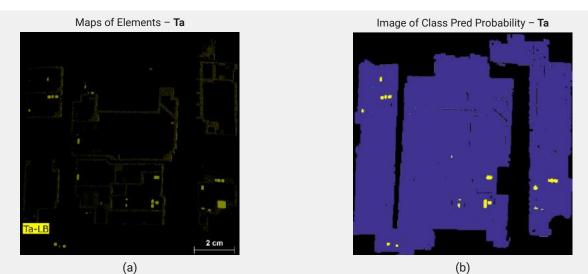
FIGURE 13: µXRF map of tantalum (Ta) element following the classical analytical approach (a) and the PLS-DA prediction modelling (b).
