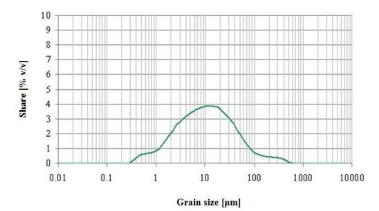
FIGURE 7: Histogram curve of particle size distribution of the waste sample.
