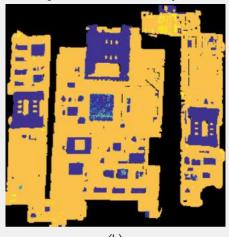
(a) (b) FIGURE 12:  $\mu XRF$  map of copper (Cu) element (a) following the classical analytical approach and as resulting from the PLS-DA prediction
