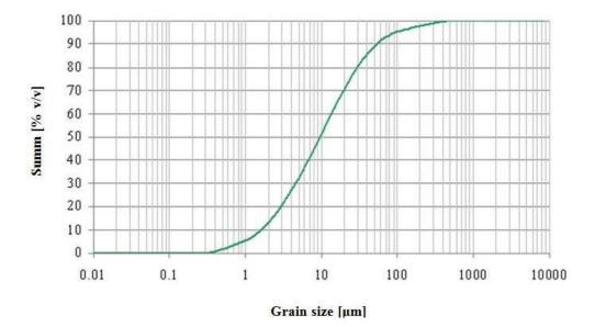
FIGURE 6: Cumulative curve of particle size distribution of the waste sample.
