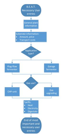
**FIGURE 1:** Flow chart of the calculation tool B.E.A.T. (Biogas installations Economic Assessment Tool).
