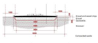
FIGURE 3: Design of the trails at Kudjape landfill.
