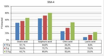
FIGURE 3: Leaching tests performed with different acids at different L/S ratios.
