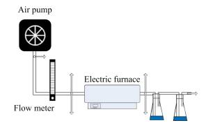
FIGURE 5: Schematic illustration of combustion experiment equipment.
