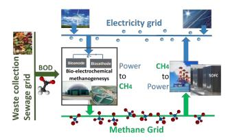
FIGURE 3: Scheme of the potential interface between the electricity and methane distribution grids, based on converting all organic waste/wastewater treatment facilities into Electromethanogenesis units.
