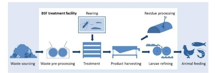
FIGURE 1: The different units of a BSF treatment system (Dortmans et al, 2017).
