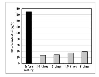
FIGURE 3: Results of chemical oxygen demand (COD) - leachate test before and after washing.
