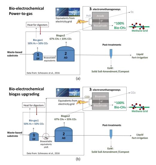
FIGURE 2: The concepts under investigation in this project: a) electromethanogenesis is used as bioelectrochemical power-to-gas system and all bioavailable equivalents yielded from dark fermentation are sent to AD methanogenesys; b) electromethanogenesis acts as bioelectrochemical biogas upgrading system and a fraction of bioavailable equivalents is sent to the bioanodic compartment, as counter-reactive.
