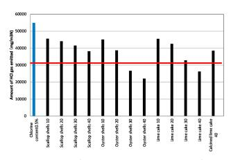
FIGURE 8: Amount of HCl gas emitted by addition ratio of single antichlors (waste).
