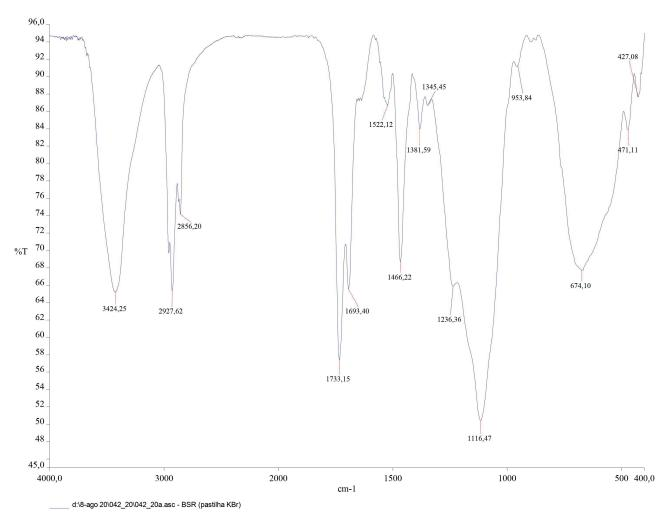
FIGURE 4: FTIR of the backsheet.
