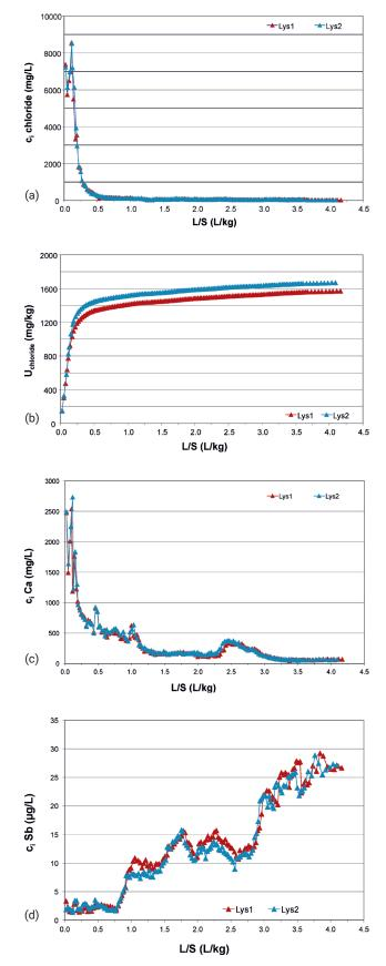
**FIGURE 1:** Results from the long-term lysimeter experiment as a function of L/S. a: Concentrations  $c_i$  of chloride. b: Cumulative release U of chloride, c: Concentrations  $c_i$  of calcium, d: Concentrations  $c_i$  of antimony.
