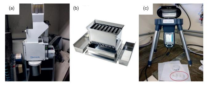
FIGURE 2: Metal content characterization (a) knife mill (b) stainless steel sample quarters (c) portable XRF analyzer and sample storage capsules for analysis, highlighted in red.
