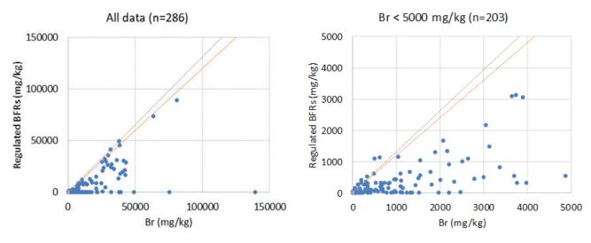
**FIGURE 1**: Regulated brominated flame retardants (R-BFRs) as a function of total bromine content (left) and the same data with  $Br \le 5,000 \text{ mg/kg}$  (right), with stoichiometric ratio R-BFRs/Br of 1.20 w/w (orange line) and 1.31 w/w (grey line).
