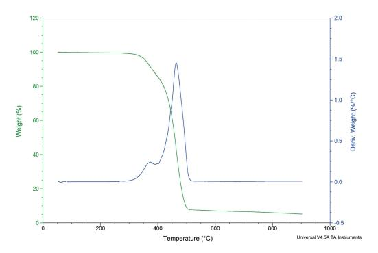
FIGURE 5: TGA of the backsheet under inert atmosphere (nitrogen gas).
