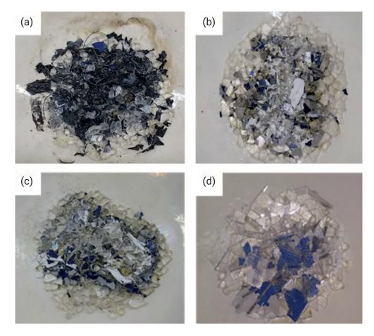
FIGURE 8: Different samples after furnace, which were kept at constant 500°C temperature for (a) 30 min (b) 60 min (c) 90 min (d) 120 min.
