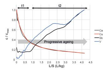
**FIGURE 3:** Concentrations of Ca, Cu, Sb, and V as a function of L/S. Assessment at the end of period t1 would allow use of the treated IBA, whereas in period t2 the concentration of Sb and V might exceed the limit values.
