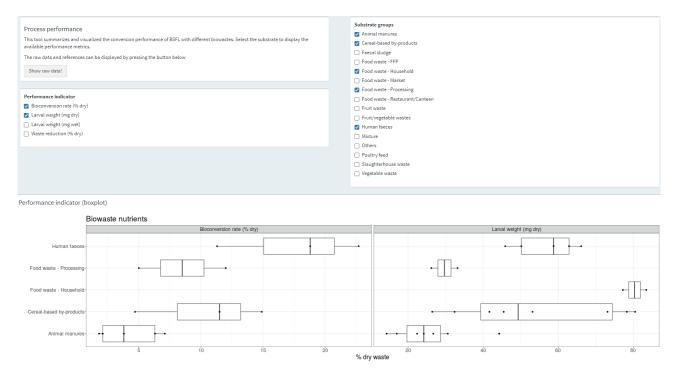
FIGURE 2: The "Conversion performance" tab of the web application summarises process performance results based on the substrate group and performance metric selected by the user. Descriptive statistics are included in a table below the boxplot (not shown in this Figure).
