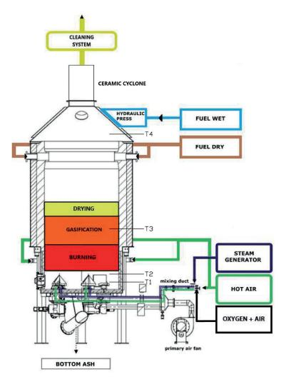
FIGURE 1: Operating scheme of the biomass gasifying unit.
