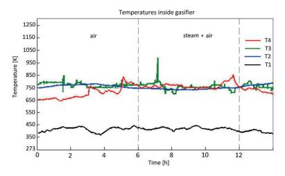
FIGURE 5: Distribution of temperatures in gasifier during air and air-steam gasification.
