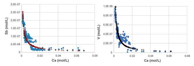
FIGURE 2: Concentration of Sb (left) and V (right) in the lysimeter experiment as a function of Ca concentration (circles). The crosses are the result of a fit with MS Excel.
