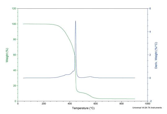
FIGURE 6: TGA of the backsheet under oxidizing atmosphere (synthetic air).
