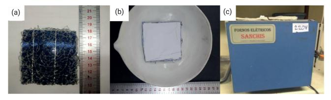
FIGURE 3: (a) Sample with dimensions 8 x 8 cm (b) Sample before heat treatment in a ceramic crucible (c) Sanchis N1100H furnace.
