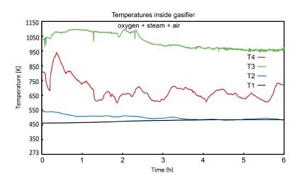
FIGURE 6: Distribution of temperatures in gasifier during oxygen-steam-air gasification.
