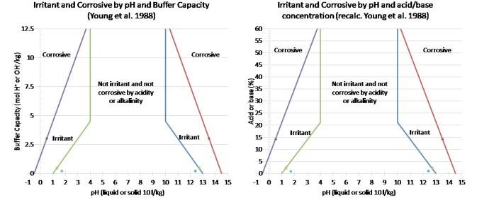
**FIGURE 3:** The pH - buffer capacity domain of irritancy and corrosiveness of Young et al. 1988, expressed in buffer capacity (left) and acid/base concentration (right). The blue points correspond to the classification of products in the CLP, and the yellow and red points to classification as irritant and corrosive by Young et al. (1988).
