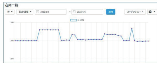
Actual image of the data management system. Data acquired by the weighing device were monitored on the cloud system.
