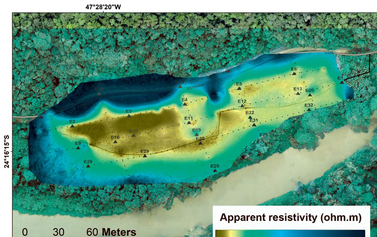
**FIGURE 8:** Geophysical results in Miracatu dump expressed in scales of electrical resistivity in the subsoil.
