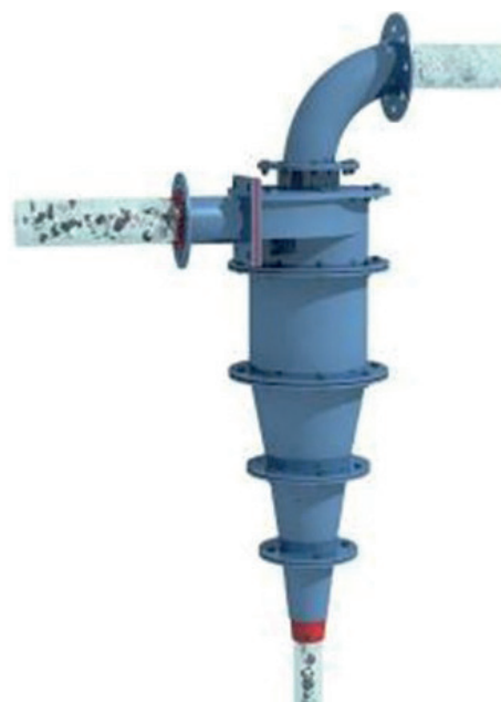
FIGURE 4: Representation of a hydro-cyclone.
