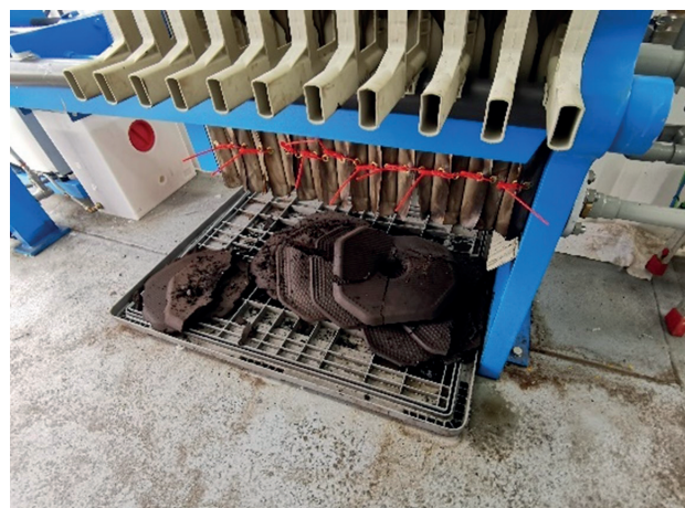
FIGURE 3: Carbonized material recovered after filtration.
