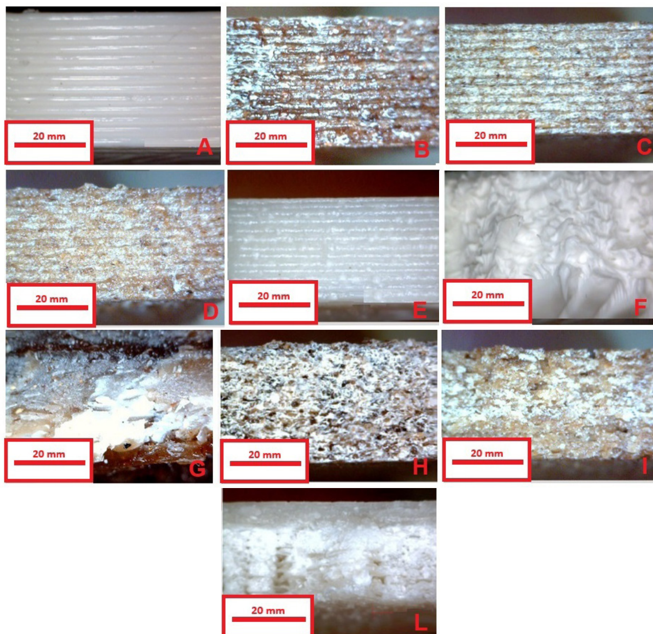
FIGURE 4: Magnified images (50x) of the 3D bars after bending test: printing surface of 100PLA (A), 90PLA/10CBSW (B), 90PLA/10OW (C), 90PLA/10LSW (D) and 90PLA/10CW (E); breaking surface after bending test of 100PLA (F), 90PLA/10CBSW (G), 90PLA/10OW (H), 90PLA/10LSW (I) and 90PLA/10CW (L).
