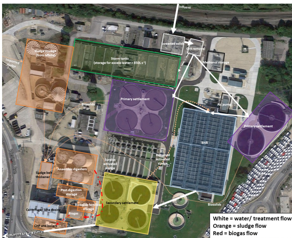
FIGURE 1: Aerial view of the Millbrook site detailing the flows of wastewater (white arrows), biosolids and activated sludge (orange dotted arrows), and biogas (red dotted arrow) between the labelled treatment areas.
