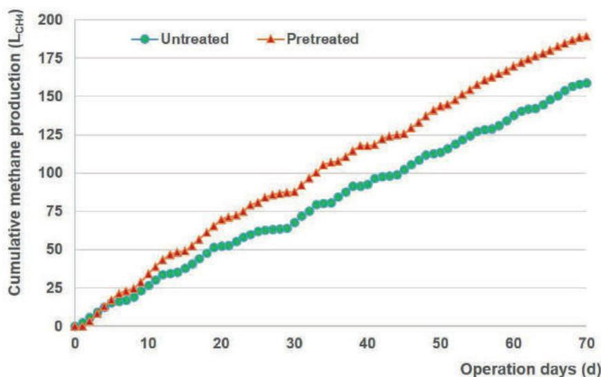
**FIGURE 3:** CH<sub>4</sub> production of untreated and pretreated solid residues during the long-term AD process (HRT 20d).
