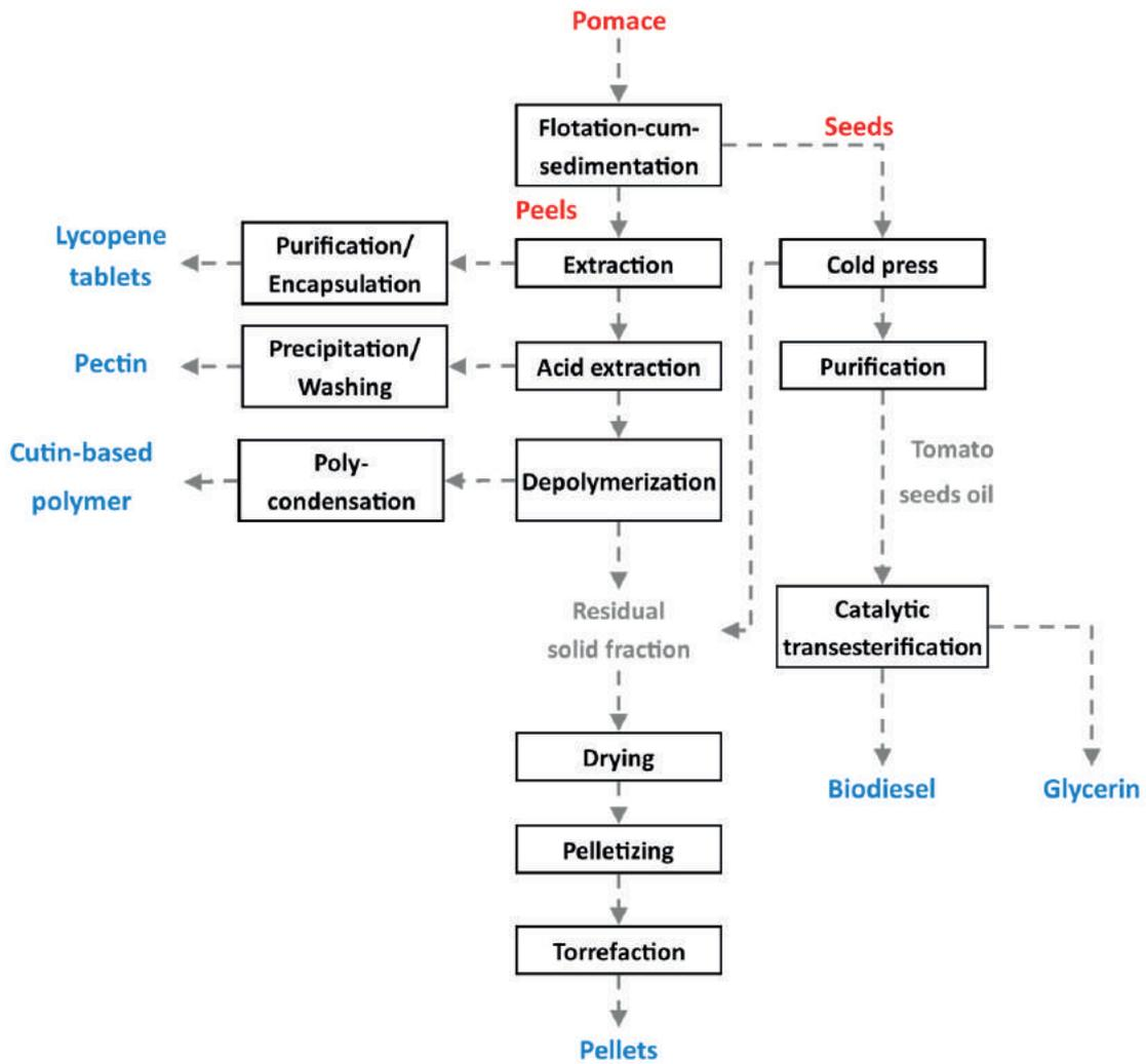
**FIGURE 1:** Biorefinery model for a full exploitation of tomato processing by-products (feedstocks are reported in red font, process units in black, intermediate materials in grey and biorefinery products in blue).
