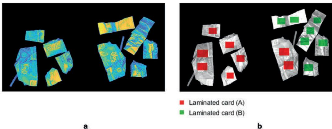
**FIGURE 7:** Laminated card particles (side A is the plastic/paper/metal/plastic side, while side B is the plastic/metal/paper/plastic side): a) concatenated hyperspectral images of the particles and b) ROIs selected on the hyperspectral images (Red: laminated card - side A, green: laminated card - side B).
