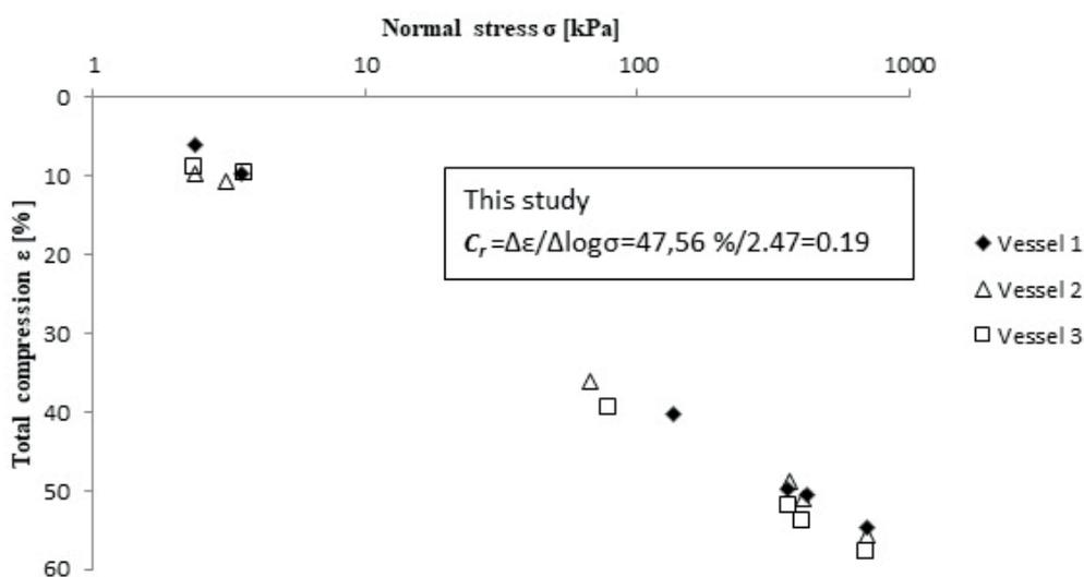
**FIGURE 7:** Total compression  $\epsilon$  [%] as function of normal stress  $\sigma$  [kPa] in log scale for the three used cylinders. The compression index  $C_r$  is defined as the slope of the curve.
