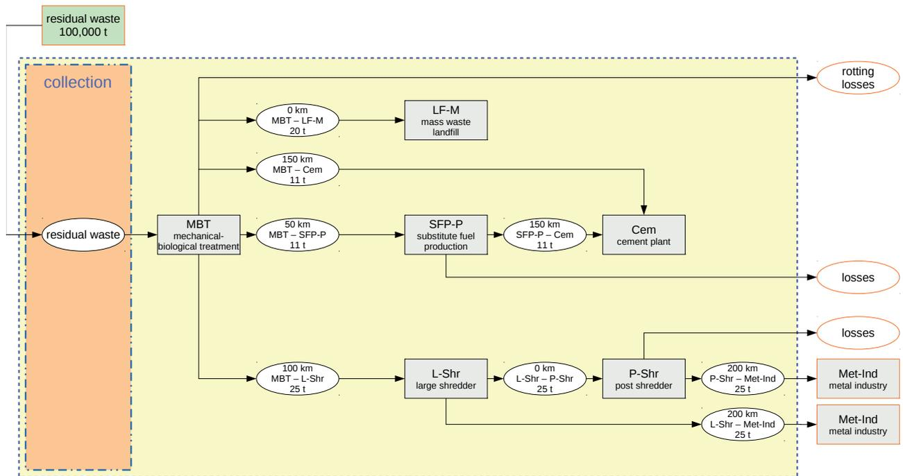
FIGURE 6: Model 3.3 - MBT + cement plant
