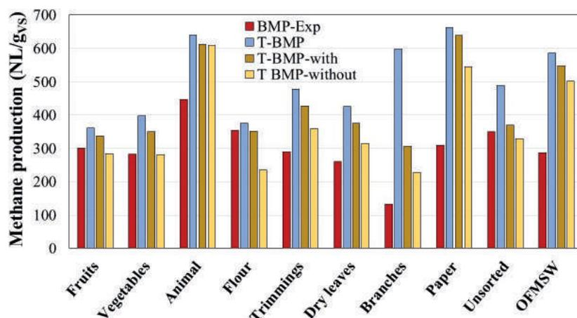
**FIGURE 4:** Methane production from OFMSW fractions after 21 days reaction. BMP-Exp (experimental); T-BMP (theoretical BMP); T-BMP-with (lignocellulosic substances); T-BMP-without (lignocellulosic substances).
