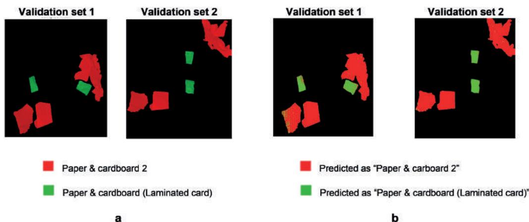
**FIGURE 11:** The validation set 1 and set 2 - “Paper & cardboard 2” - “Paper & cardboard (Laminated card)” classification: actual classes (a) and classes predicted by the PLS-DA model. Fragments were correctly classified by the two-class PLS-DA model as comparing the actual classes to the prediction map.
