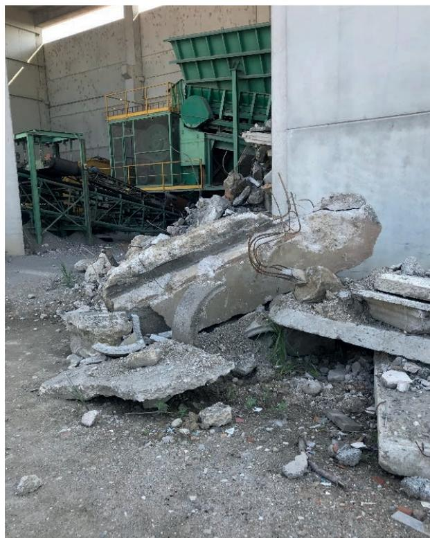
**FIGURE 5:** CDW large elements with unsuitable size for direct crushing.
