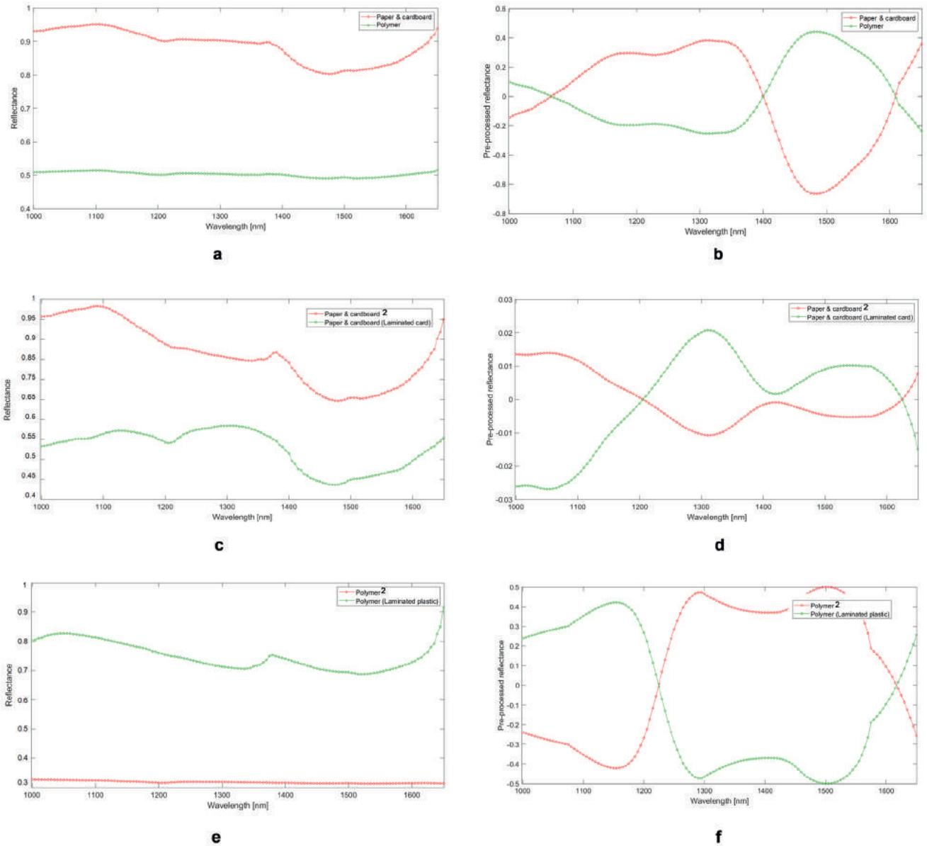
**FIGURE 10:** “Paper & cardboard” - “Polymer” calibration set: grand-average of raw reflectance spectra (a) and pre-processed spectra (b). “Paper & cardboard 2” and “Paper & cardboard (Laminated card)” calibration set: grand-average of raw reflectance spectra (c) and pre-processed spectra (d). “Polymer 2” and “Polymer (Laminated plastic)”: grand-average of raw reflectance spectra (e) and pre-processed spectra (f).
