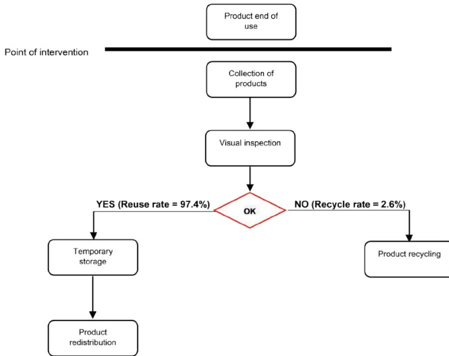
**FIGURE 6:** Project protocol and processes including the interventions made using ISB model (I: temporary storage; S: collection and inspection of products; B: products are redirected and made to pass through the system which recovers items with residual reuse value).
