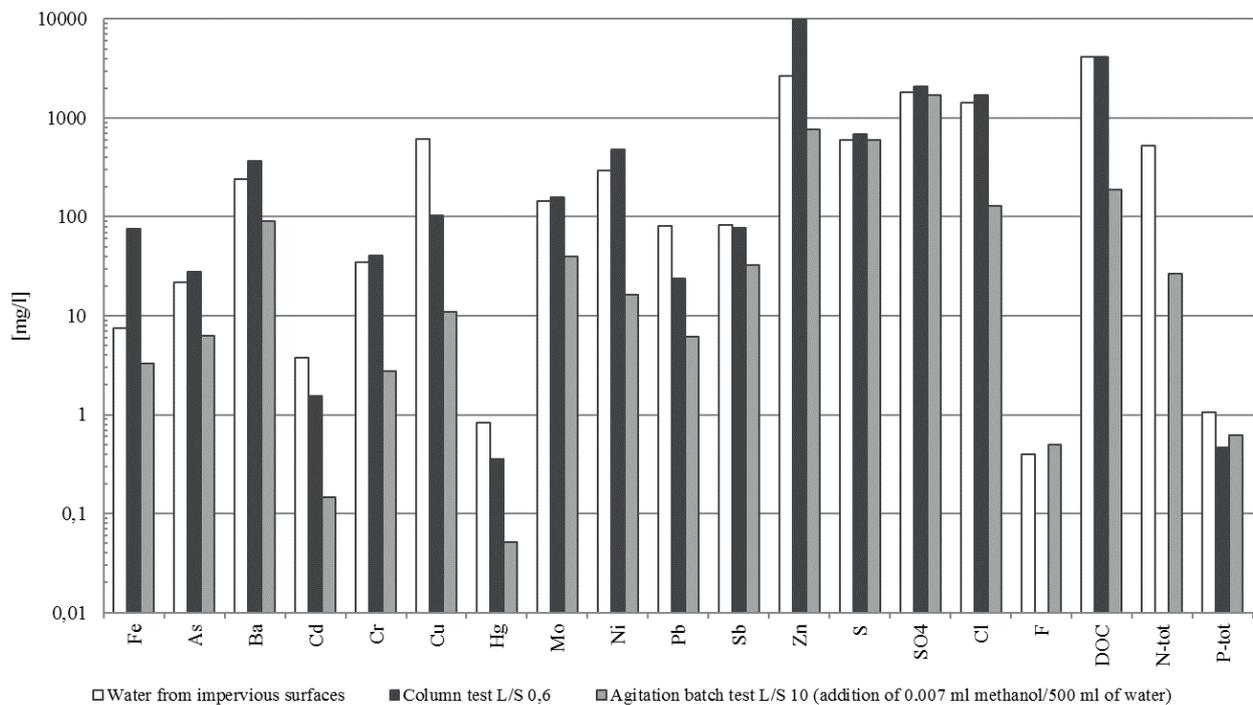
**FIGURE 5:** Concentration of elements in leachate from USFMS; water from impervious surfaces (1 sample, filtered), leachate from column test at L/S ratio 0.6 (3 samples, non-filtered) and leachate from agitation batch test at L/S ratio 10 (3 samples, filtered).
