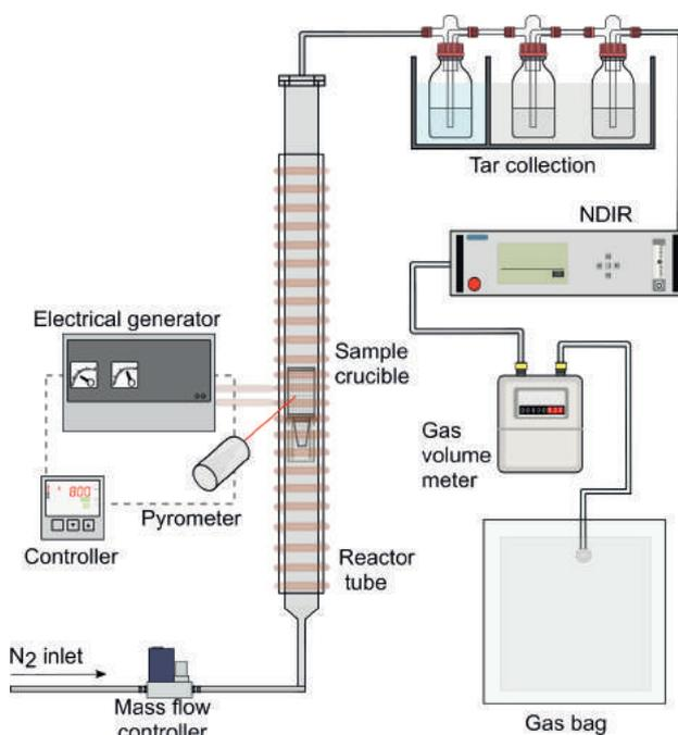
**FIGURE 1:** Schematic diagram of the lab scale device.
