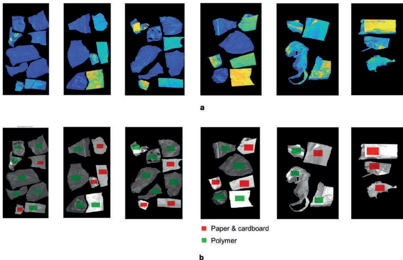
**FIGURE 6:** “Calibration set”: hyperspectral images (a) and selected ROIs of “Paper & cardboard” and “Polymer” (b). Red: Paper & cardboard, green: Polymer.
