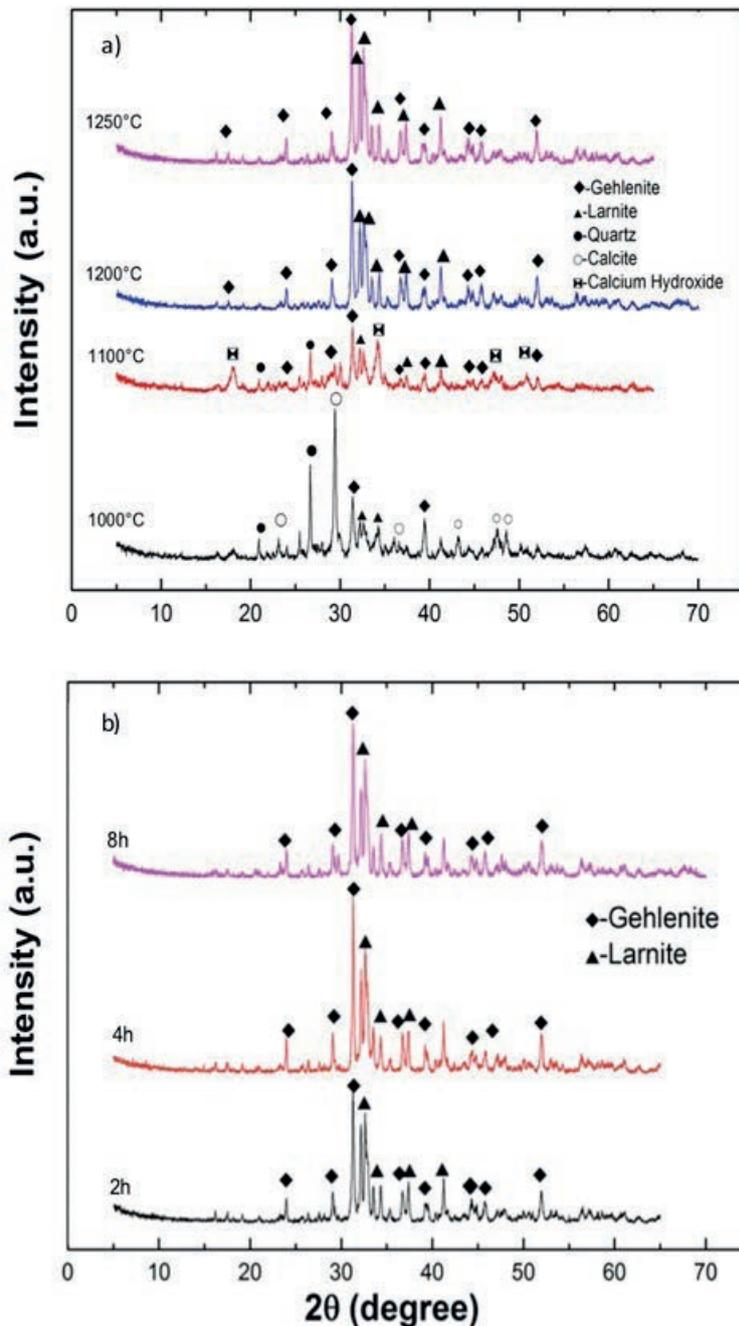
**FIGURE 5:** a) XRD analysis of CDW A6 sample treated at different temperature and same duration of 2 hours each; b) A6 at the highest temperature (1250°C) and different durations (2 to 8 h).
