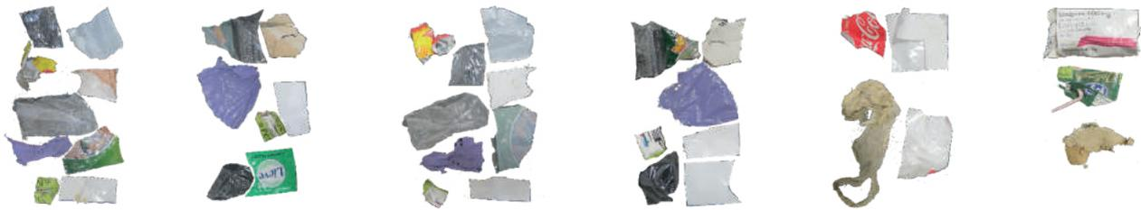
**FIGURE 2:** Digital images of particles included in the calibration set to build a model able to recognize paper-based fragments from polymer-based particles.
