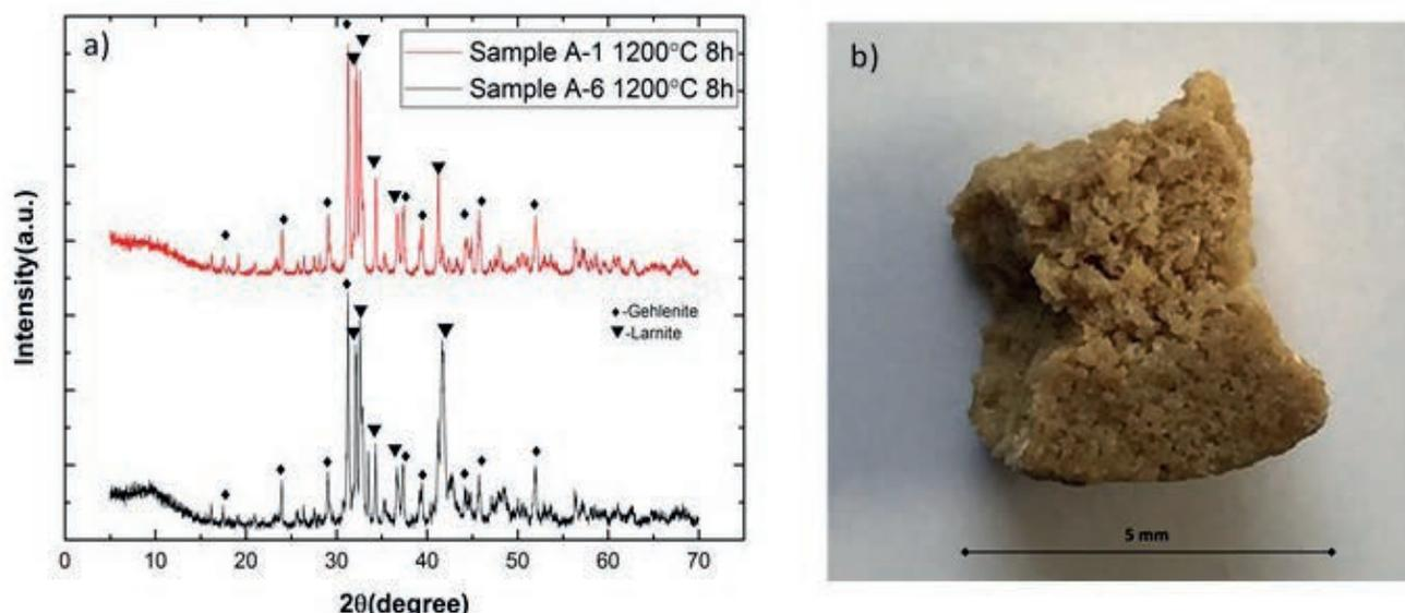
**FIGURE 6:** (a) Comparison of XRD data between the samples A1 and A6 after thermal treatment at the same temperature (1200°C) and duration (8h). (b) The porous material produced at high temperature from the CDW thermal treatment.
