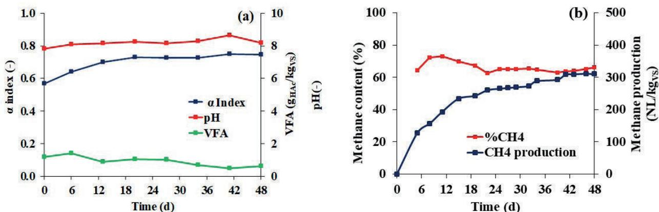
FIGURE 3: Behaviour of reactor operational parameters during inoculum adaptation.
