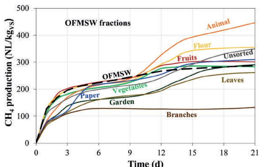
FIGURE 3: Methane production from OFMSW fractions.
