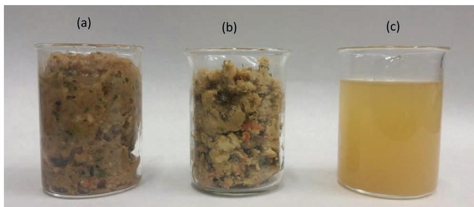
**FIGURE 1:** The Food waste (a), the solid residue (b) and the liquid extract (c) obtained after pretreatment and centrifugation.
