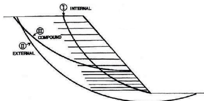
FIGURE 1: Failure modes for reinforced soil slopes.
