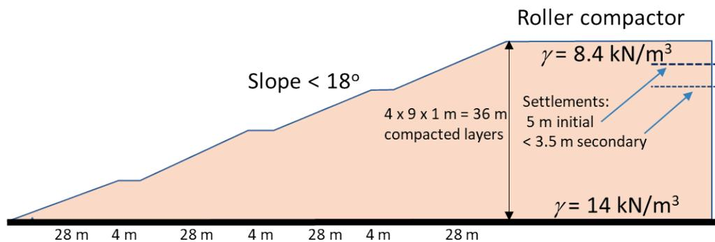
**FIGURE 13:** Proposed principle outline of a landfill with 36 compacted layers of 1 m with approximate initial and secondary settlements. Slopes should feature horizontal terraces every 5 to 10 meters to increase stability.
