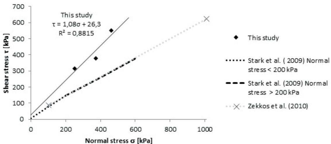
**FIGURE 6:** Shear strength envelope for USFMS and results from previous studies. R2 denotes the coefficient of determination in the linear regression formula.
