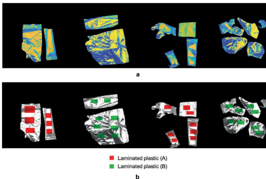
**FIGURE 8:** Laminated plastic particles (side A is the plastic/metal side, while side B is the metal/plastic): a) concatenated hyperspectral images of the particles and b) ROIs selected on the hyperspectral images (Red: laminated plastic - side A, green: laminated plastic - side B).
