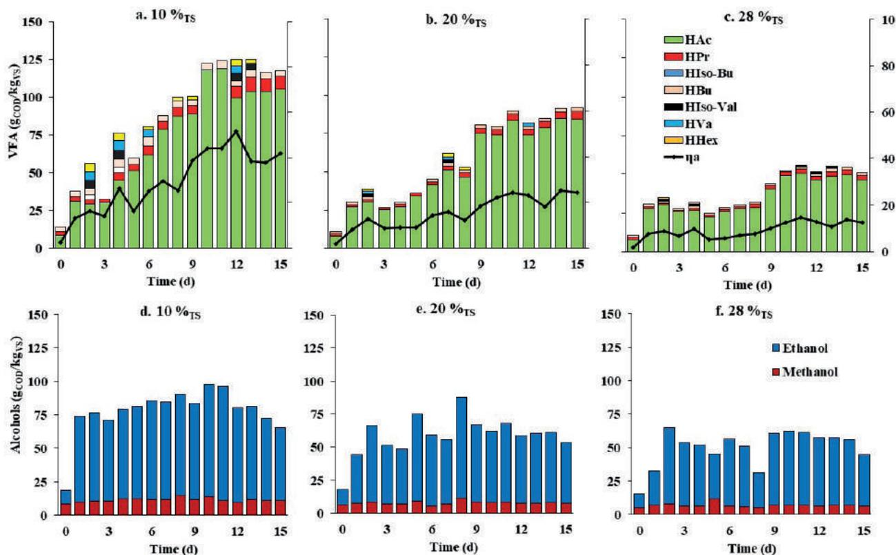
**FIGURE 2:** VFA and alcohol production, and acidification rate ( $\eta_a$ ). HAc (acetic acid), HPr (propionic acid), HIsoBu (isobutyric acid), HBu (butyric acid), HIso-Val (isovaleric acid), HVa (valeric acid), HHex (hexanoic acid).
