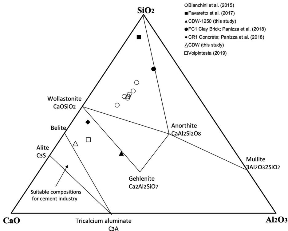
**FIGURE 4:** Ternary diagram describing the system CaO–Al<sub>2</sub>O<sub>3</sub>–SiO<sub>2</sub> (wt%). Triangles are our CDW study composition (empty starting material, full after thermal treatment at 1250°C, circles are data from Bianchini et al. (2015) and full square from Favaretto et al. (2017). A clay brick and a concrete composition (Panizza et al. 2018) are reported as comparison.
