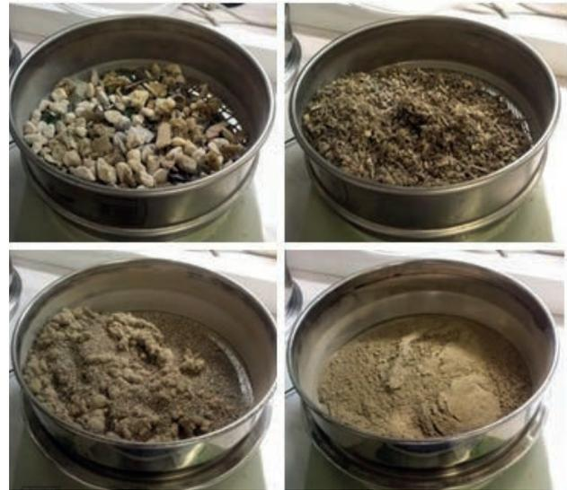
**FIGURE 12:** Photos from dry sieving. Above: to the left waste > 8 mm, to the right waste > 2mm. Below: to the left waste > 0.5 mm, to the right waste > 0.063 mm.
