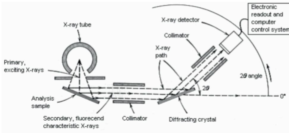
FIGURE 3: WD XRF instrumentation picture.
