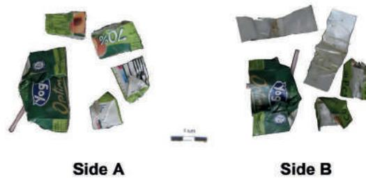
**FIGURE 4:** Digital images of laminated card particles. Side A: 5 fragments with the plastic/paper/metal/plastic side exposed and Side B: 4 fragments with the plastic/metal/paper/plastic side exposed.
