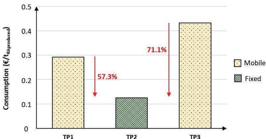
FIGURE 6: TP consumption per tonne of RAs produced.
