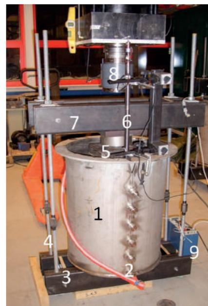
**FIGURE 3:** Test rig. (1) Compression vessel; (2) Outlet connected to hose; (3) Foundation; (4) Threaded rods; (5) Load cell and metal plate; (6) Linear variable differential transformer (LVDT); (7) Head beam; (8) Servo controlled cylinder, and (9); Driver for LVDT.
