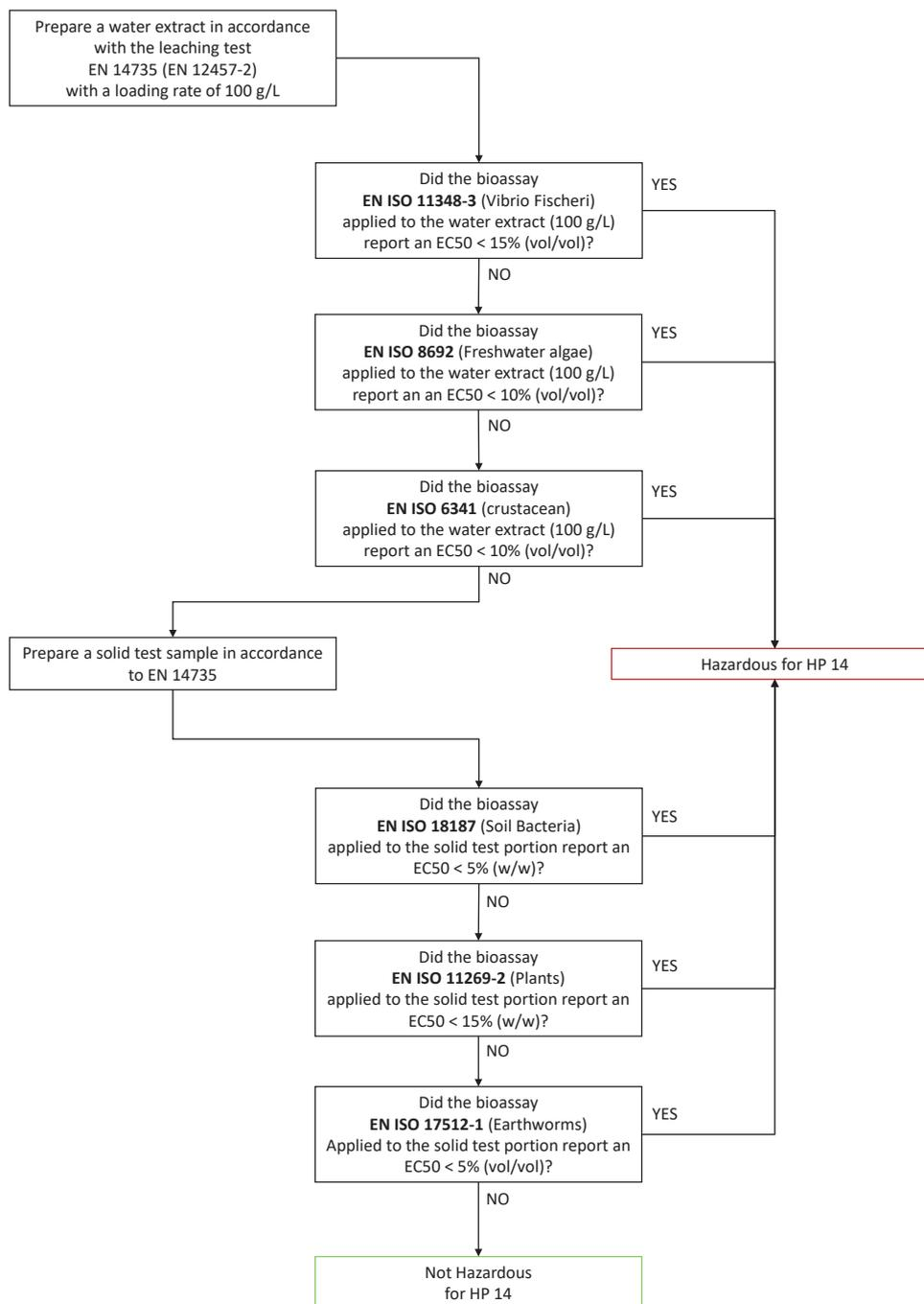
**FIGURE 3:** “Waste-based approach.” Proposed decision tree for HP 14 classification of waste according to the international standards proposed in Pandard and Römbke, (2013) and the classification limits established in Hennebert (2018, 2019).
