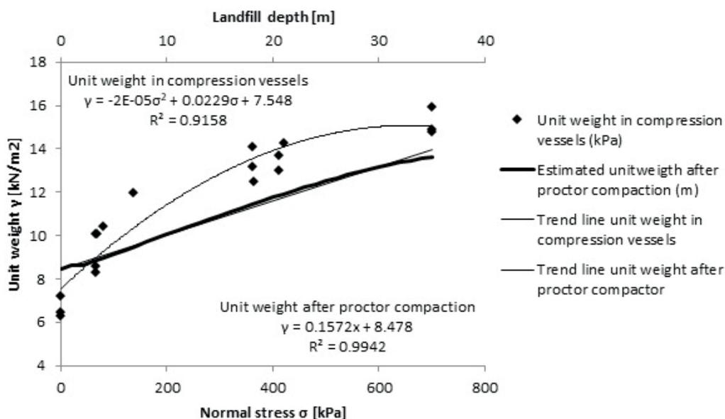
**FIGURE 8:** Unit weight in the three compression vessels as function of compaction stress and a trend line indicating mean value for the three vessels. Calculated unit weight as function of landfill depth after compaction with 40 kPa.
