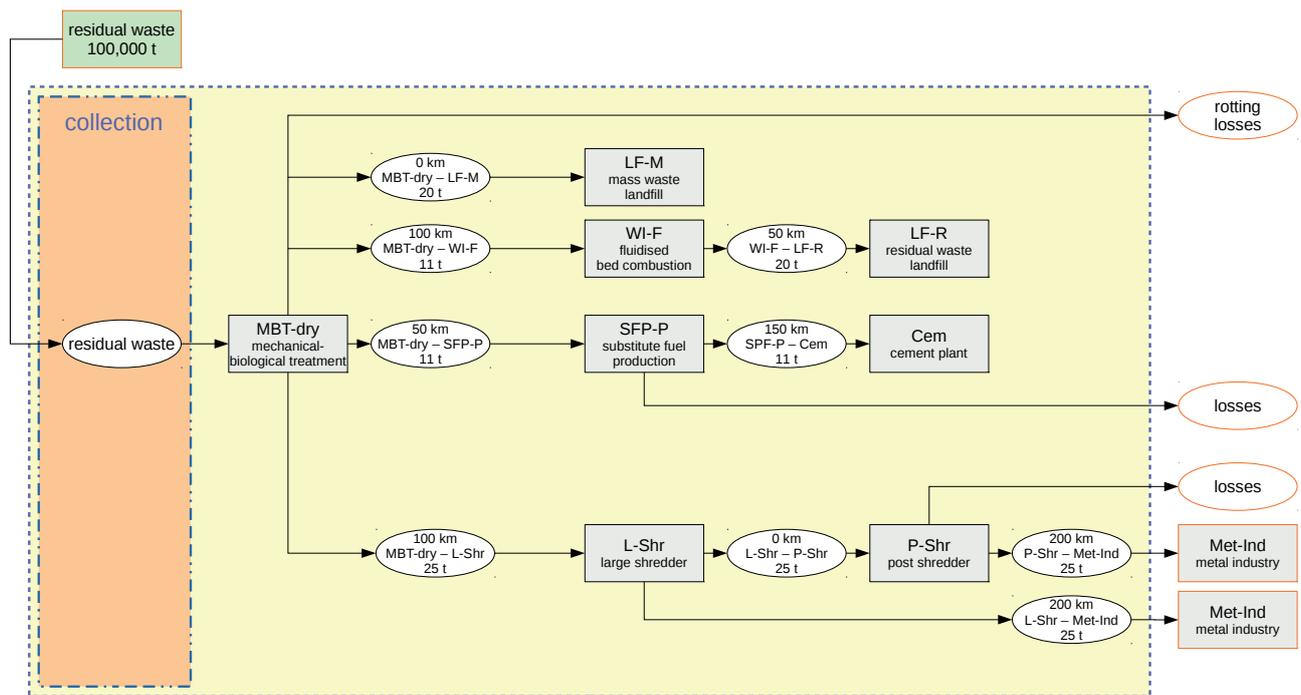
FIGURE 7: Model 3.4 - MBT with dry stabilization + incineration + cement plant.
