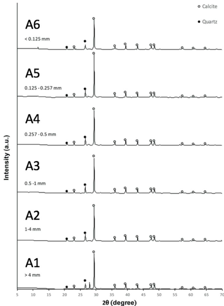
**FIGURE 3:** XRD mineralogical composition of CDW different granulometries. Notes: full circles are Quartz; empty circles are Calcite; grain-size intervals in mm are reported.
