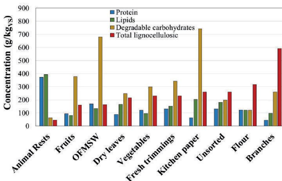
**FIGURE 2:** Comparison of bromatological characteristics in the separated fractions. The fractions are organized in ascending concentration of total lignocellulosic substances.
