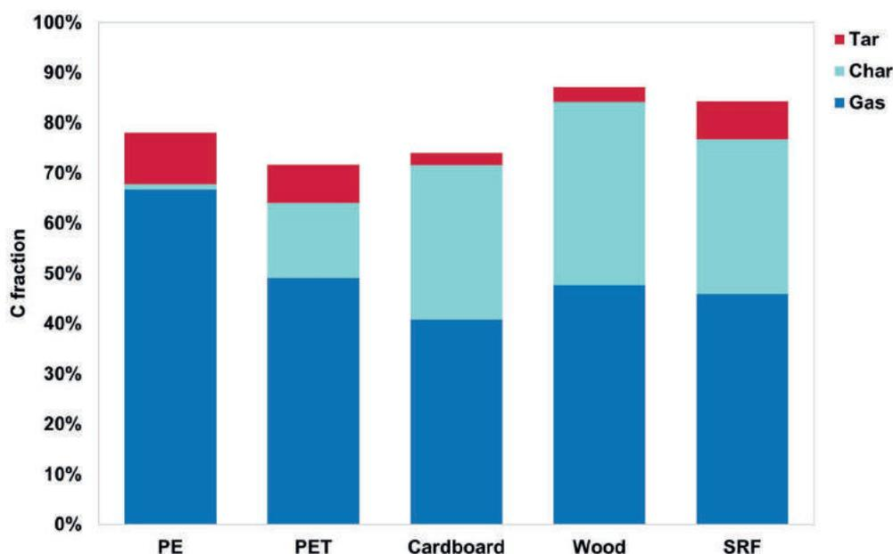
FIGURE 2: Carbon distribution from SRF and its components to pyrolysis products at 800°C.
