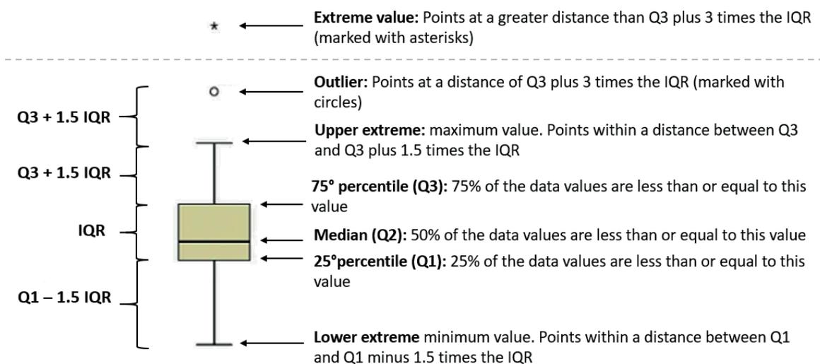
FIGURE 1: Structure of the box-plot chart.
