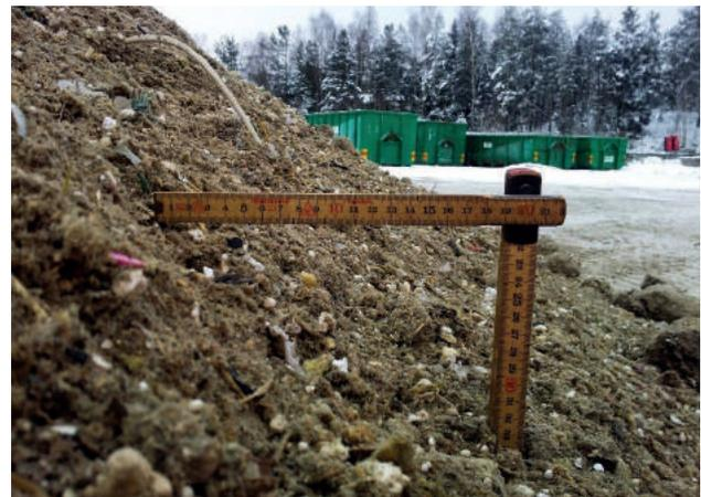
**FIGURE 2:** The USFMS during sampling and measuring of the angle of repose.
