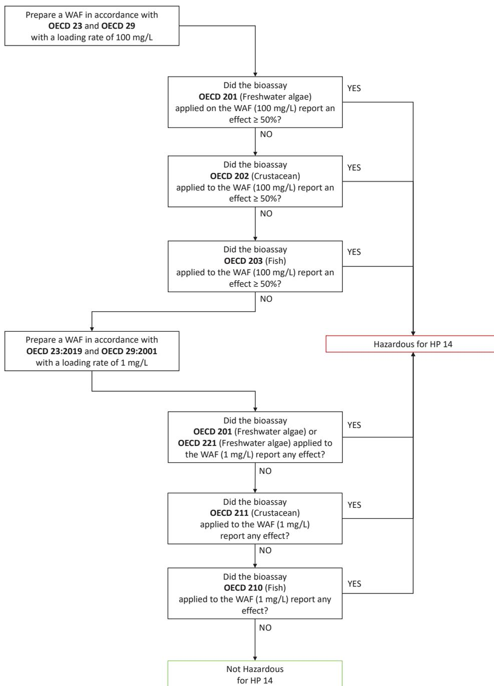
**FIGURE 2:** “CLP-based approach.” Proposed decision tree for HP 14 classification of waste with methods validated for CLP. WAF: Water Accommodated Fractions. OECD 23: Guidance Document on Aquatic Toxicity Testing of Difficult Substances and Mixtures; OECD 29: Guidance document on transformation/dissolution of metals and metal compounds in aqueous media; OECD 201, 202, 203, 210 and 211: see Table 2.
