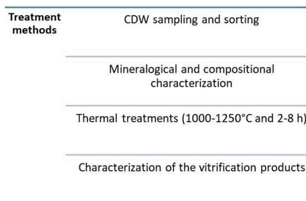
**FIGURE 1:** Methodological chart showing the sequence of treatments on CDW.
