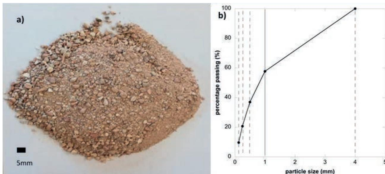
**FIGURE 2:** (a) CDW sample before sieving; (b) Rosin Rammler particle size distribution.
