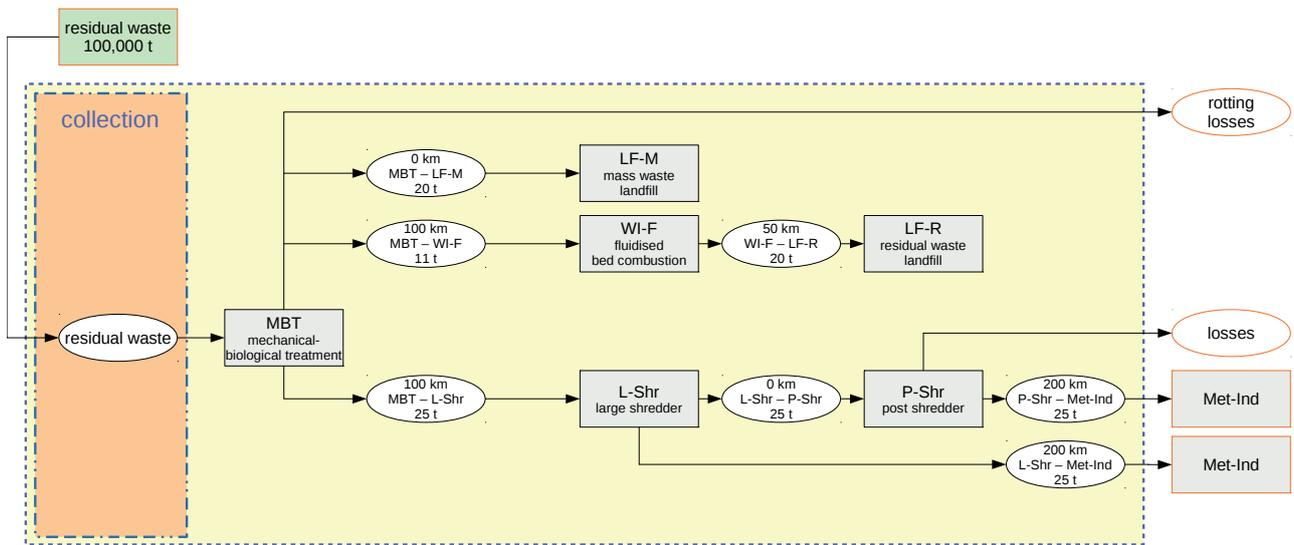
FIGURE 4: Model 3.1 - MBT + incineration.
