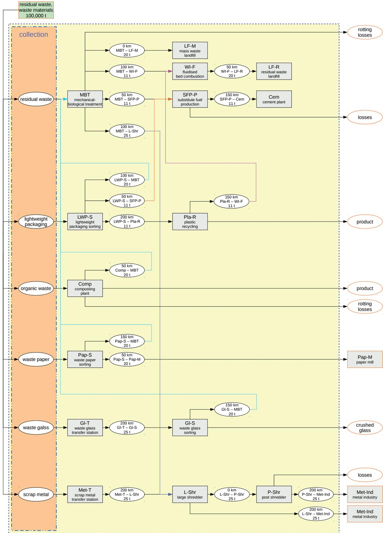
FIGURE 8: Model 4 - Improved separate collection.
