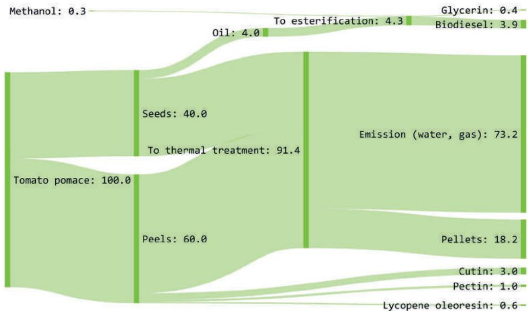
**FIGURE 2:** Mass balance for tomato by-products in tonnes.
