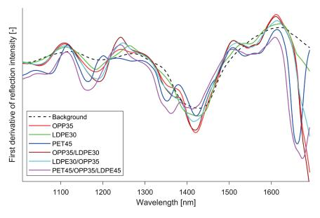
**FIGURE 2**: Mean spectra of background, OPP35, LDPE30, PET45, OPP35/LDPE30, LDPE30/OPP35 and PET45/OPP35/LDPE30. (Sample name is material with thickness, e.g. OPP35/LDPE30 is two-layer sample with one OPP layer with a thickness of 35  $\mu$ m and one LDPE Layer with a thickness of 30  $\mu$ m, the OPP layer is exposed to NIR sensor).
