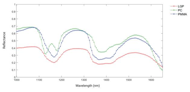
FIGURE 7: Raw spectra of virgin "PC" and "PMMA" polymers compared with LGP spectral signatures.
