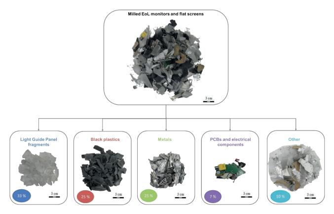
FIGURE 1: Diagram of the analyzed sample: product resulting from a milling line of a WEEE recycling plant and main material categories resulting from manual sorting. The composition (weight %) of the different main material categories is reported.
