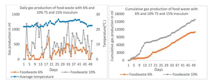
FIGURE 8 AND 9: Daily and Cumulative Gas production in trial 3 Semi-continuous reactors.
