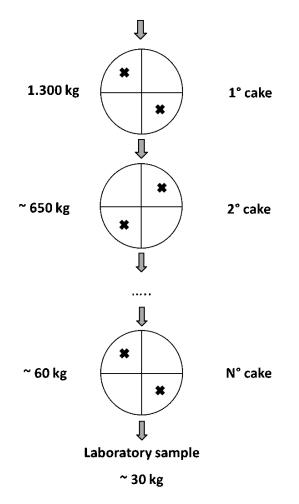
FIGURE 3: Quartering procedure for the preparation of the final laboratory sample (derived from EN 15002:2013).
