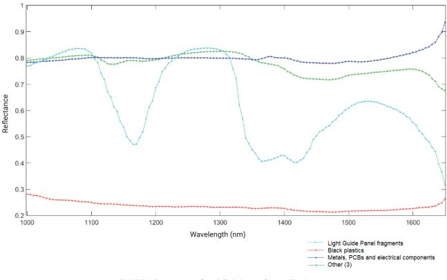
FIGURE 4: Raw spectra of modelled classes from calibration set.
