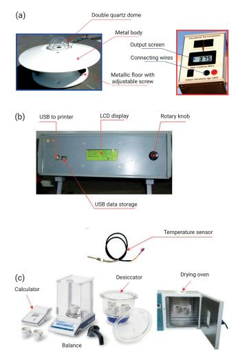
**FIGURE 3:** Photographs of measuring instruments. (a) Eppley PSP pyranometer with output screen. (b) Data acquisition and RTD temperature sensor. (c) Drying oven and balance apparatus.
