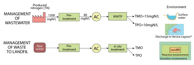
FIGURE 5: Graph parallel between the management of sewage forwarded to a depuration plant and management of wastes forwarded to landfill. WWTP, Wastewater treatment plant. \*Limits for discharge into the Venice lagoon laid down in Ministerial Decree 30/7/99.
