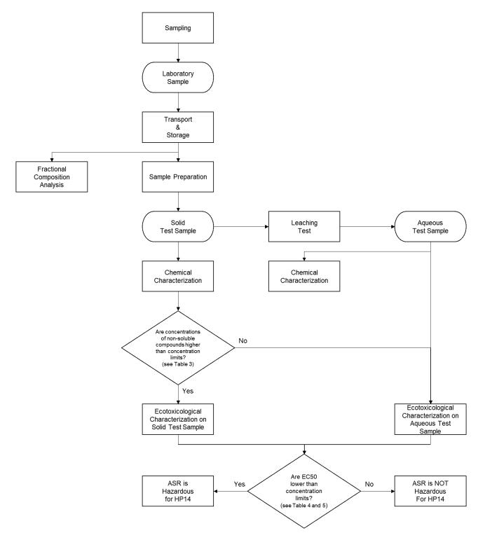
FIGURE 1: Stepwise procedure for HP14 classification of Automotive Shredder Residues (ASR).
