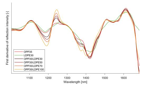
FIGURE 4: Mean spectra of samples with OPP 35  $\mu$ m and LDPE 30, 50, 70 and 100  $\mu$ m.
