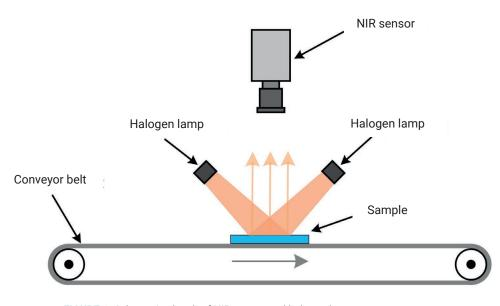
FIGURE 1: Schematic sketch of NIR sensor and halogen lamps arrangement.
