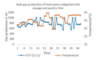
FIGURE 10: Daily gas production with co-digestion of food waste, sewage sludge, and poultry.
