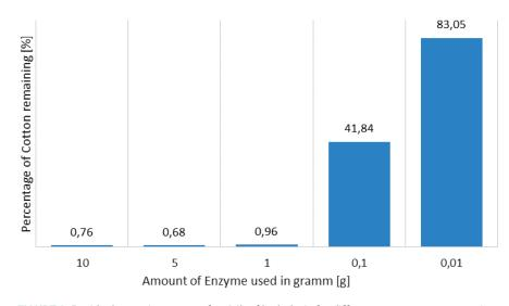
FIGURE 2: Residual mass in percent after 24h of hydrolysis for different enzyme conecentrations.
