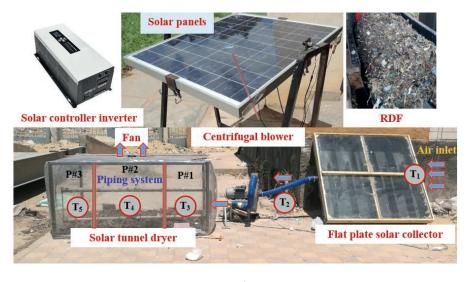
FIGURE 2: Photograph of experimental set-up.
