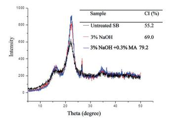
FIGURE 1: Diffractograms and crystallinity index (CI) of untreated SB and solid fractions resulting from pretreatment with 3.0% NaOH (one-stage pretreatment) and 3.0%NaOH+0.3%MA (onestage NaOH pretreatment followed by the second-stage maleic acid pretreatment) respectively.
