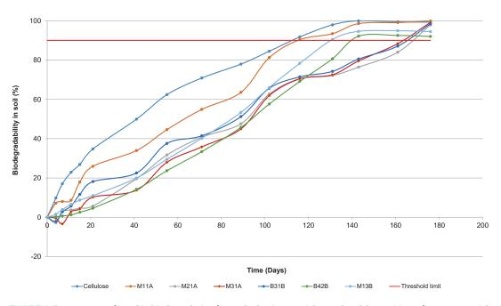
FIGURE 2: Percentages of aerobic biodegradation for each plastic material tested and the positive reference material.
