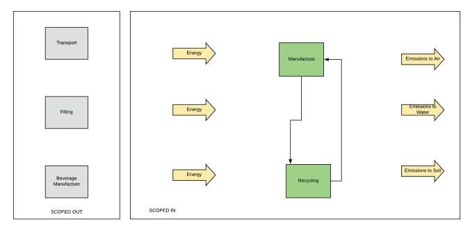
FIGURE 2: Hypothetical product system and scoped out processes for beverage packaging made from 100% recycled materials.
