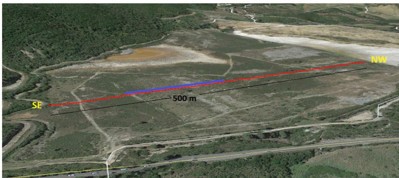
**FIGURE 1:** The San Giorgio mine tailings basin (southwestern Sardinia – Italy). The red and blue lines indicate, respectively, the position of the gravity and the shallow reflection profiles.
