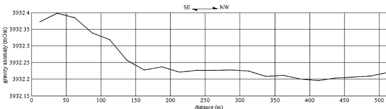
**FIGURE 2:** Gravity anomaly measured along the profile crossing the mine tailings basin of San Giorgio as shown in Figure 1.
