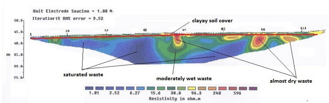
FIGURE 7: Electrical resistivity tomography on an old disposal site hosting demolition rubble in southern Sardinia - Italy.
