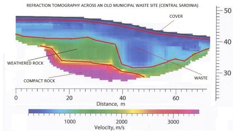
**FIGURE 6:** Refraction tomography (compressional waves) along a profile crossing the old municipal waste site located as shown in Figure 5.
