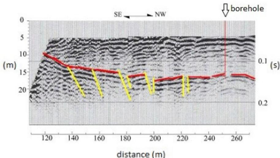
**FIGURE 3:** Depth-converted seismic section partially superimposed to the gravity profile as shown in Figure 1. The bottom of the basin, as well as several faults affecting the latter, are clearly identifiable.
