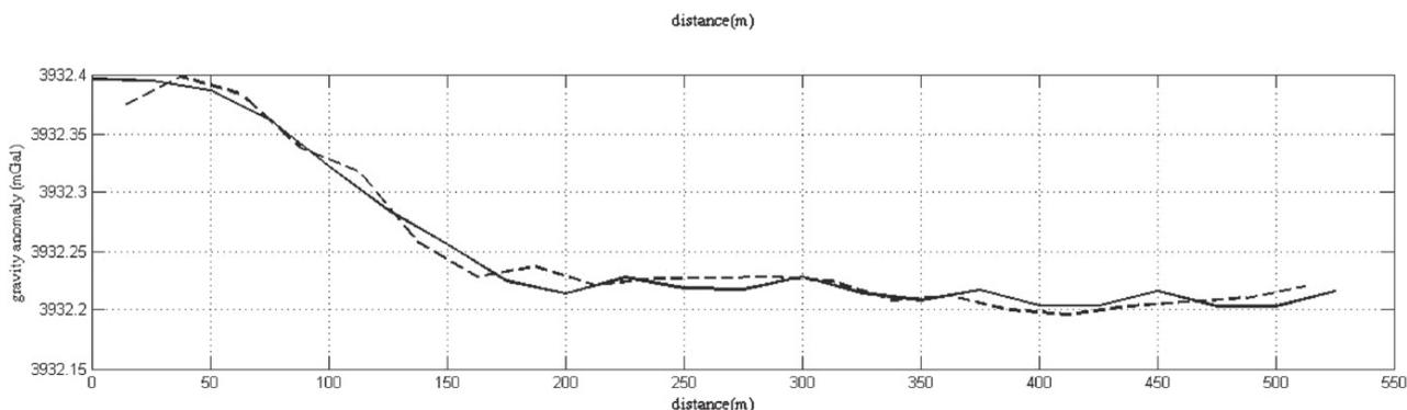
**FIGURE 4:** Best fit between the measured (solid line) and computed gravity anomaly (dashed line). This result was obtained for a density contrast of - 360 kg/m<sup>3</sup> between the waste and the host rock.
