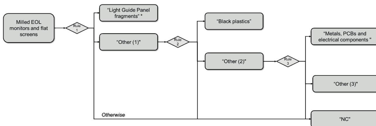
**FIGURE 3:** Flow-chart of the implemented hierarchical classification modelling. \*Starting from Light Guide Panel (LGP) fragments, a classification procedure was applied to perform polymers (PC and PMMA) identification.
