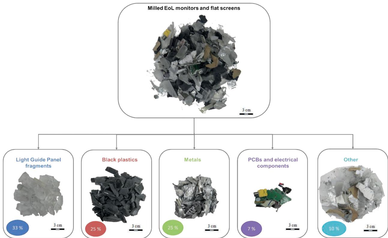
**FIGURE 1:** Diagram of the analyzed sample: product resulting from a milling line of a WEEE recycling plant and main material categories resulting from manual sorting. The composition (weight %) of the different main material categories is reported.
