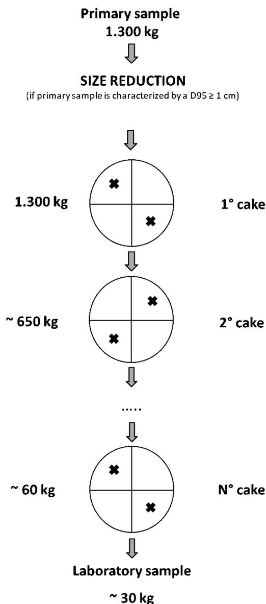
**FIGURE 3:** Quartering procedure for the preparation of the final laboratory sample (derived from EN 15002:2013).
