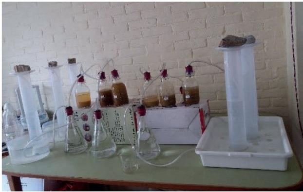
**FIGURE 2:** Picture of a batch reactors.
