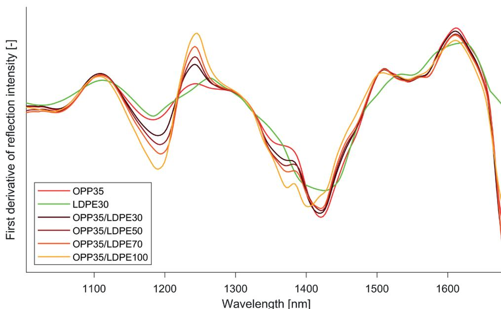
FIGURE 4: Mean spectra of samples with OPP 35  $\mu\text{m}$  and LDPE 30, 50, 70 and 100  $\mu\text{m}$ .
