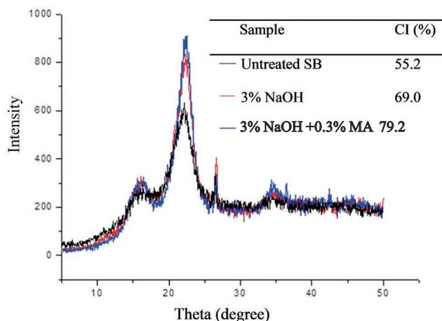
**FIGURE 1:** Diffractograms and crystallinity index (CI) of untreated SB and solid fractions resulting from pretreatment with 3.0% NaOH (one-stage pretreatment) and 3.0%NaOH+0.3%MA (one-stage NaOH pretreatment followed by the second-stage maleic acid pretreatment) respectively.
