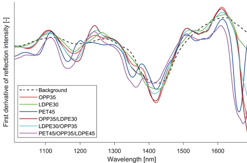
**FIGURE 2:** Mean spectra of background, OPP35, LDPE30, PET45, OPP35/LDPE30, LDPE30/OPP35 and PET45/OPP35/LDPE30. (Sample name is material with thickness, e.g. OPP35/LDPE30 is two-layer sample with one OPP layer with a thickness of 35  $\mu\text{m}$  and one LDPE Layer with a thickness of 30  $\mu\text{m}$ , the OPP layer is exposed to NIR sensor).
