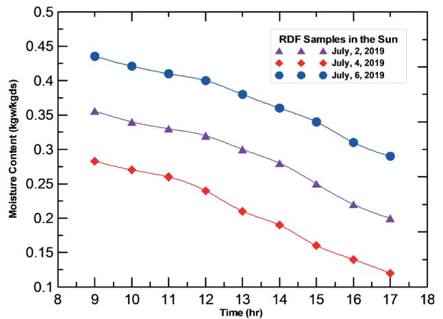
**FIGURE 9:** Variations in RDF moisture content with time for samples dried in the sun on three days when the experiment was conducted in July 2019.
