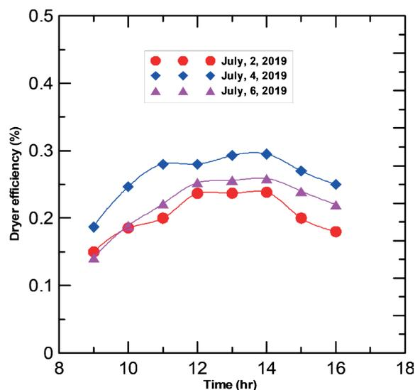
**FIGURE 11:** Variation in dryer efficiency with local time on three days when the experiment was conducted in July 2019 at air mass flow rate of 0.02 kg/s.
