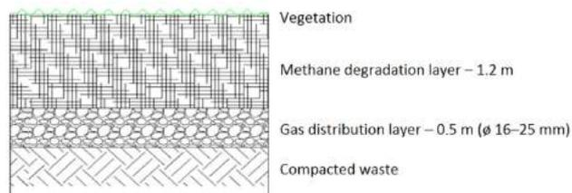
FIGURE 1: Design of the cover layer at Kudjape landfill.
