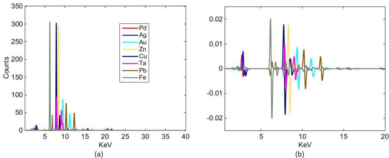
**FIGURE 6:** Raw (a) and pre-processed spectra (b), as resulting from the sequential application of the functions: Normalize (1-Norm, Area = 1), Baseline, Smoothing (order: 0, window: 5 pt, incl only, tails: polyinterp), 1st Derivative (order: 2, window: 7 pt, incl only, tails: polyinterp) and Mean Center.
