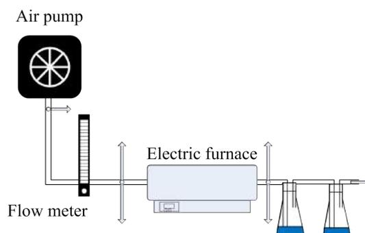
**FIGURE 5:** Schematic illustration of combustion experiment equipment.
