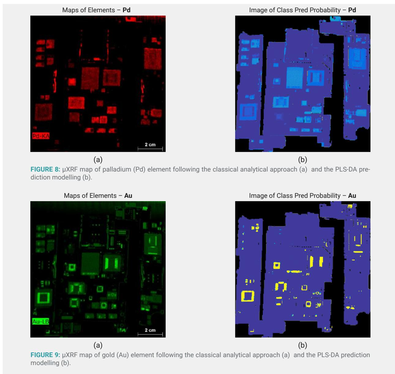
**FIGURE 8:**  $\mu$ XRF map of palladium (Pd) element following the classical analytical approach (a) and the PLS-DA prediction modelling (b).**FIGURE 9:**  $\mu$ XRF map of gold (Au) element following the classical analytical approach (a) and the PLS-DA prediction modelling (b).
