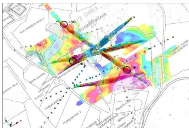
**FIGURE 5:** Electrical conductivity cross sections from 3D ERT profiles and total magnetic anomaly 2D map data with realized drill holes D1-D3 (sampling points). Interpreted bedrock topography of gravity profiles is visualized in the picture as coloured circles. In all the data the red colours show the high and blue colours show the low values.
