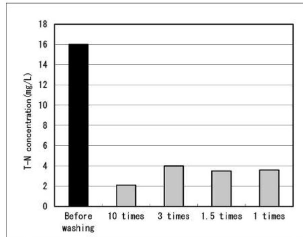
**FIGURE 4:** Results of total nitrogen (T-N) - leachate test before and after washing.
