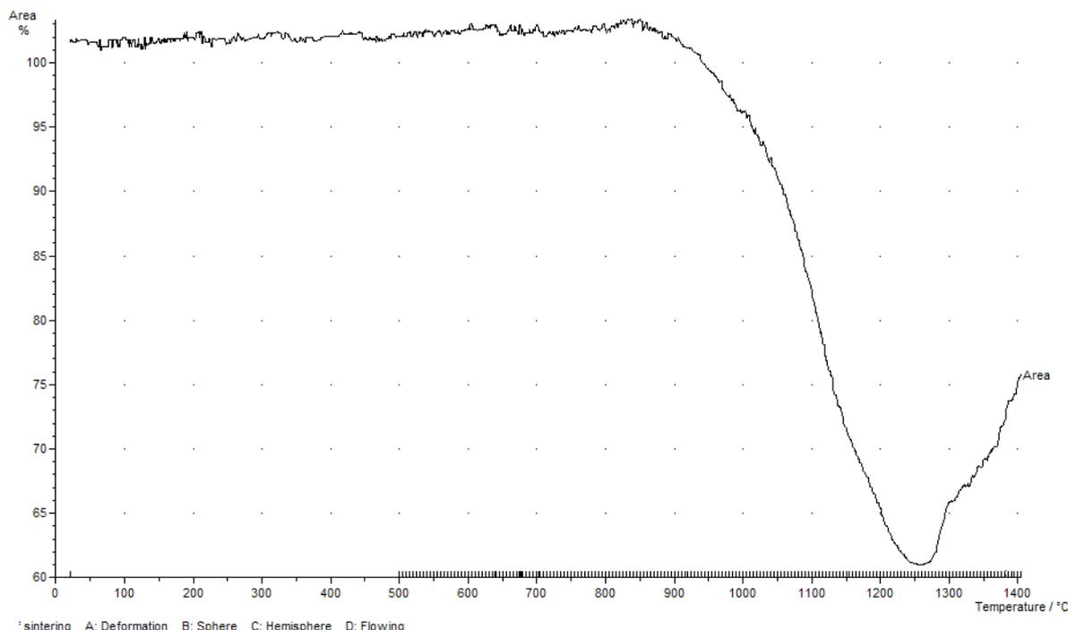
FIGURE 3: Curve showing the changes in sample profile area [in %] in line with measurements taken under the heating microscope.
