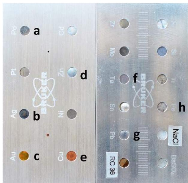
**FIGURE 2:** Digital image representing the acquired standard calibration elements: a: palladium, b: silver, c: gold, d: zinc, e: copper, f: tantalum, g: lead and h: iron.
