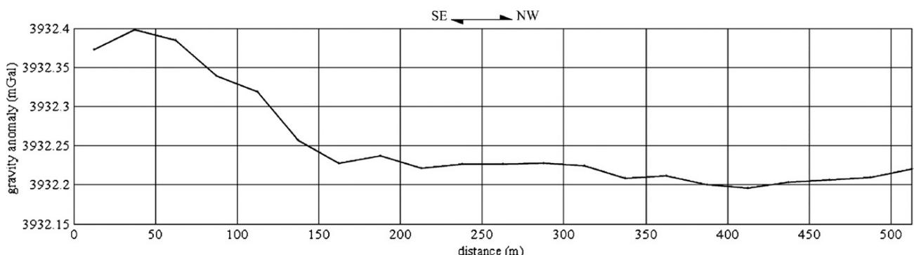
**FIGURE 2:** Gravity anomaly measured along the profile crossing the mine tailings basin of San Giorgio as shown in Figure 1.
