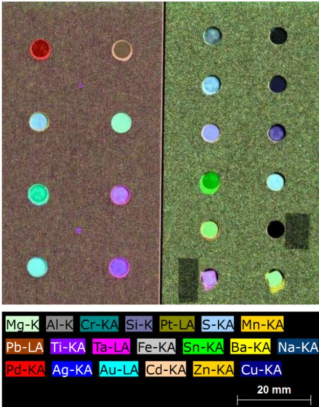
**FIGURE 5:** Elements hyper-maps of the calibration standards.
