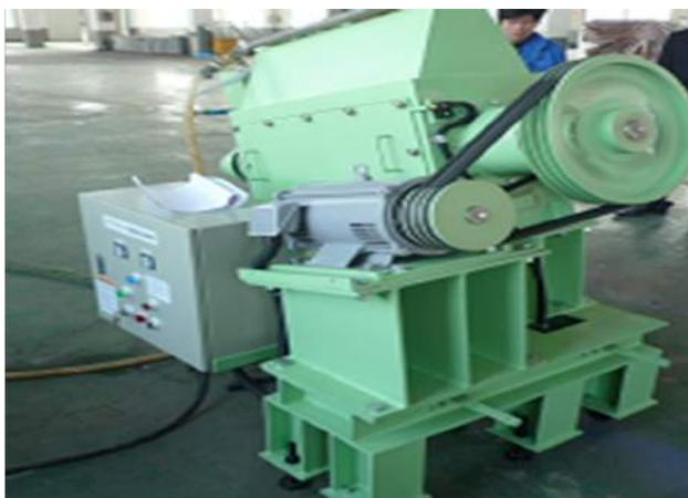
**PHOTO 1:** Rotary washer for second washing.
