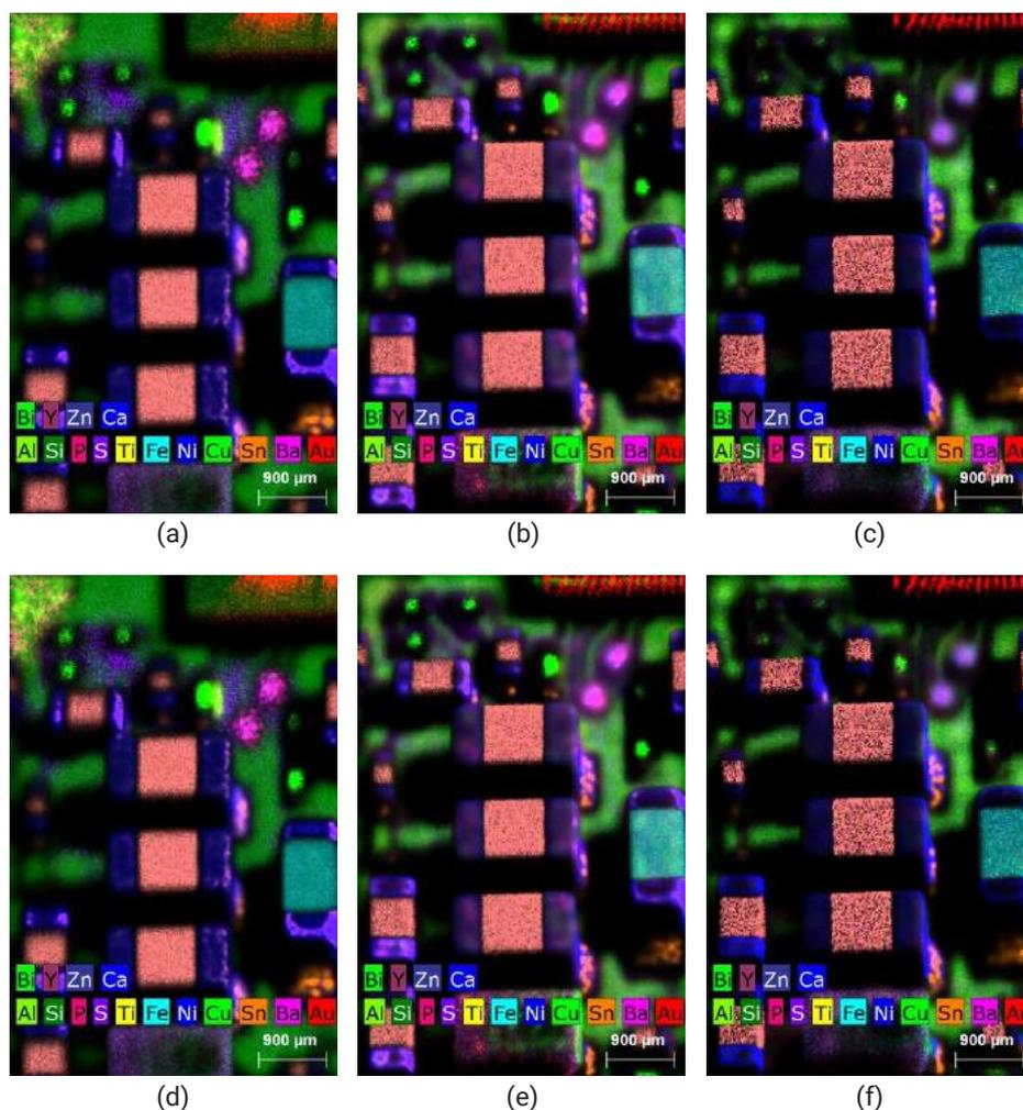
**FIGURE 3:** Hyper-maps of the elements detected by  $\mu$ XRF without filtering (a) and utilizing a Al100 (b) and a Al630 (c) filters, respectively. Detail of the distribution of gold and silicon without filtering (d) and utilizing a Al100 (e) and a Al630 (f) filters.
