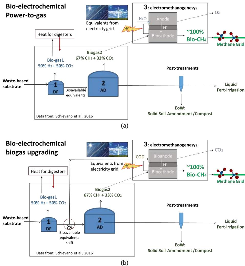
**FIGURE 2:** The concepts under investigation in this project: a) electromethanogenesis is used as bioelectrochemical power-to-gas system and all bioavailable equivalents yielded from dark fermentation are sent to AD methanogenesis; b) electromethanogenesis acts as bioelectrochemical biogas upgrading system and a fraction of bioavailable equivalents is sent to the bioanodic compartment, as counter-reactive.
