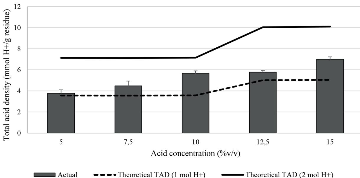
**FIGURE 7:** Total acid density (TAD) of PHR obtained at 5 to 15% v/v acid concentration, 8 mL/g SSR, 95°C for 120 minutes (theoretical TAD was calculated based on the amount of hydrolysates left in the residue).
