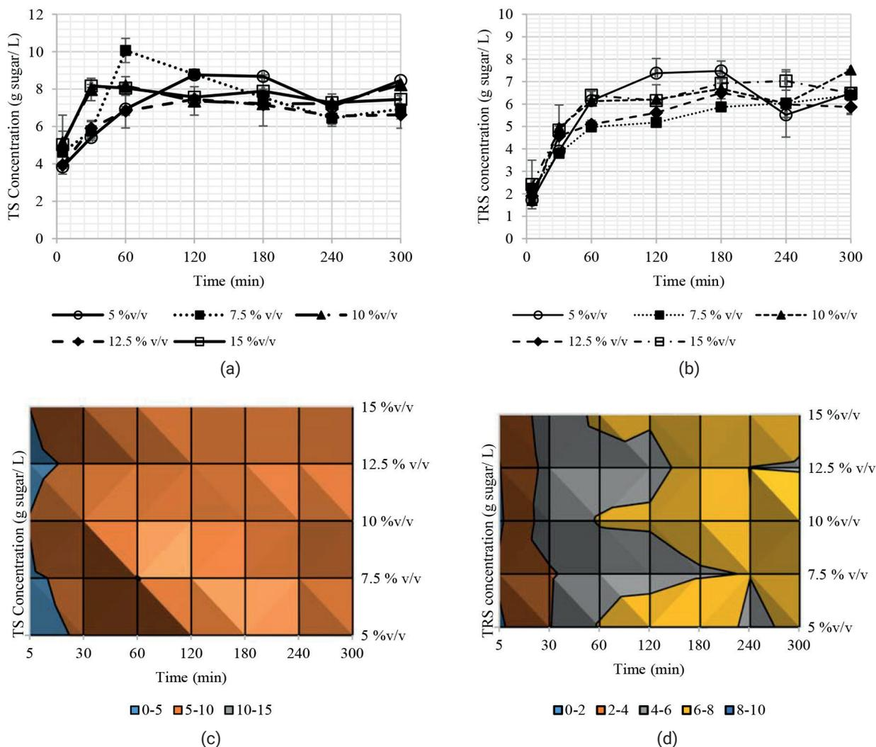
**FIGURE 2:** Sugar yields during hydrolysis at 95°C and SSR of 8 mL/g (a and c) total sugar (TS) yield versus time (b and d) total reducing sugar (TRS) versus time (This figure is to be printed in black and white in the printed version but colored in the online version).
