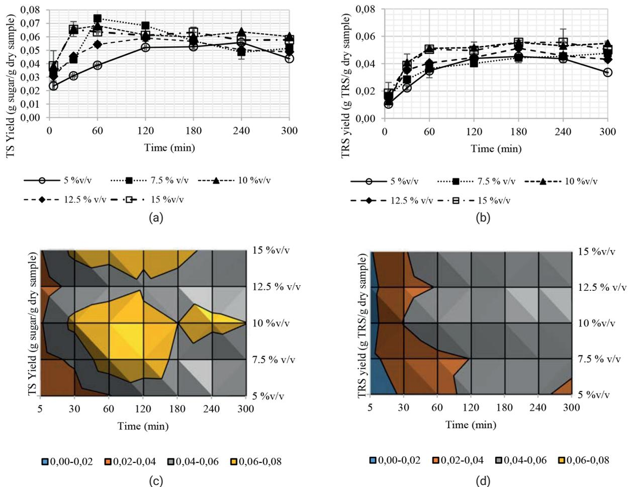
**FIGURE 1:** Sugar yields during hydrolysis at 95°C and SSR of 8 mL/g (a and c) total sugar (TS) yield versus time (b and d) total reducing sugar (TRS) versus time (This figure is to be printed in black and white in the printed version but colored in the online version).
